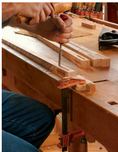
For chopping, a spacer keeps the work off the vise jaw. The pounding could damage the vise. The best support is on the benchtop itself, right over a leg.
