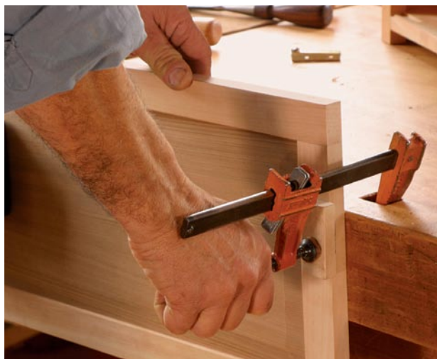
Hold wide workpieces on edge. The vise screw prevents a wide piece from going all the way through the vise (right). A clamp seated in a dog hole provides extra support (above).
