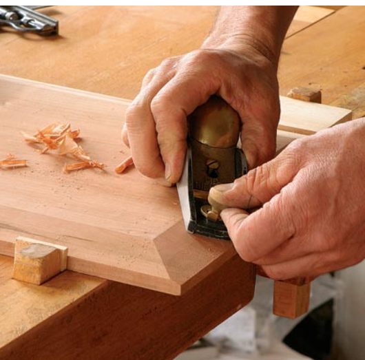
A secure grip for cross-grain work. The end vise allows you to clamp a panel across its width for tasks such as planing a bevel on the end.
