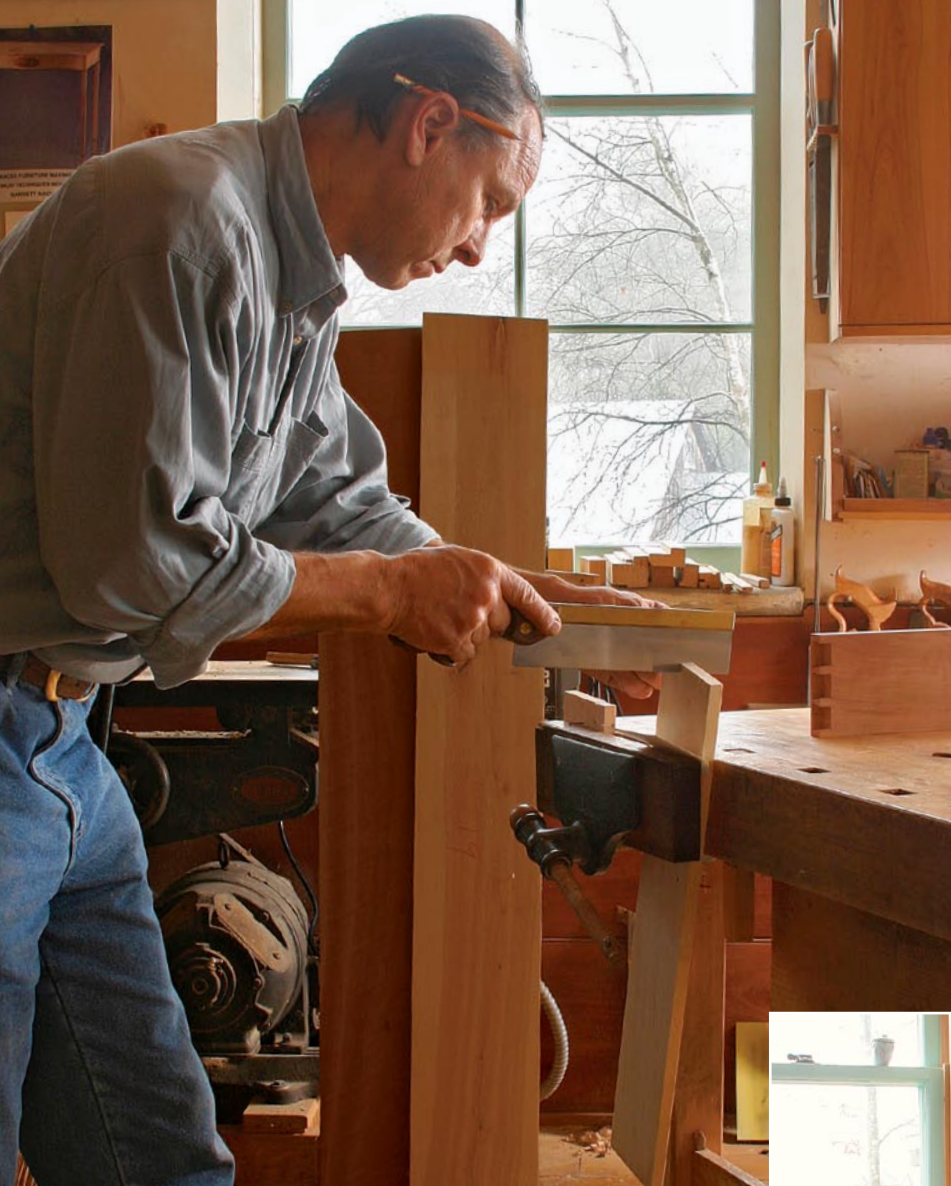
Hold work vertically for sawing dovetails or planing end grain. A scrap piece of similar thickness, clamped in the opposite side of the vise, prevents the vise from racking.
