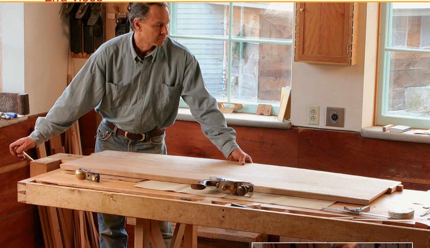
An end vise holds work flat. Aligned with a row of dog holes, this vise has a wide capacity. It can hold smaller work and pieces nearly as large as the benchtop. It's ideal for smoothing a tabletop.
