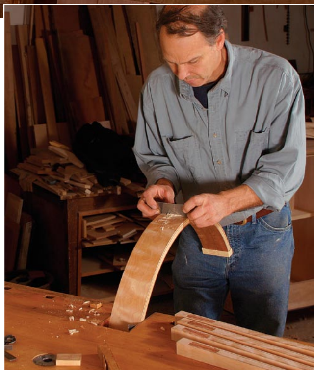
An end vise also handles awkward shapes. Pieces like this curved table apron can be held securely for scraping or other tasks.
