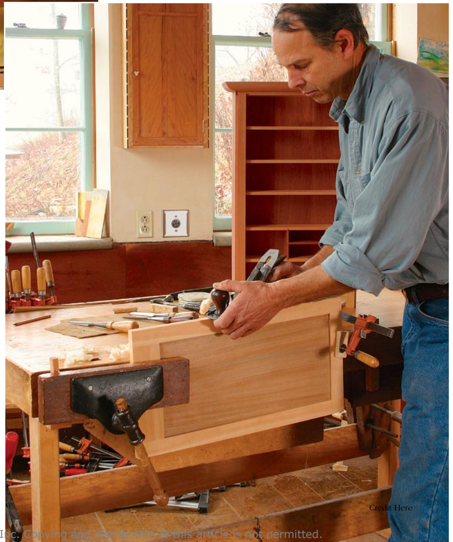
Hold wide workpieces on edge. The vise screw prevents a wide piece from going all the way through the vise (right). A clamp seated in a dog hole provides extra support (above).
