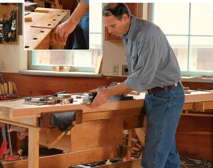
Secure long boards on edge. A block clamped in the tail vise supports the opposite end.
