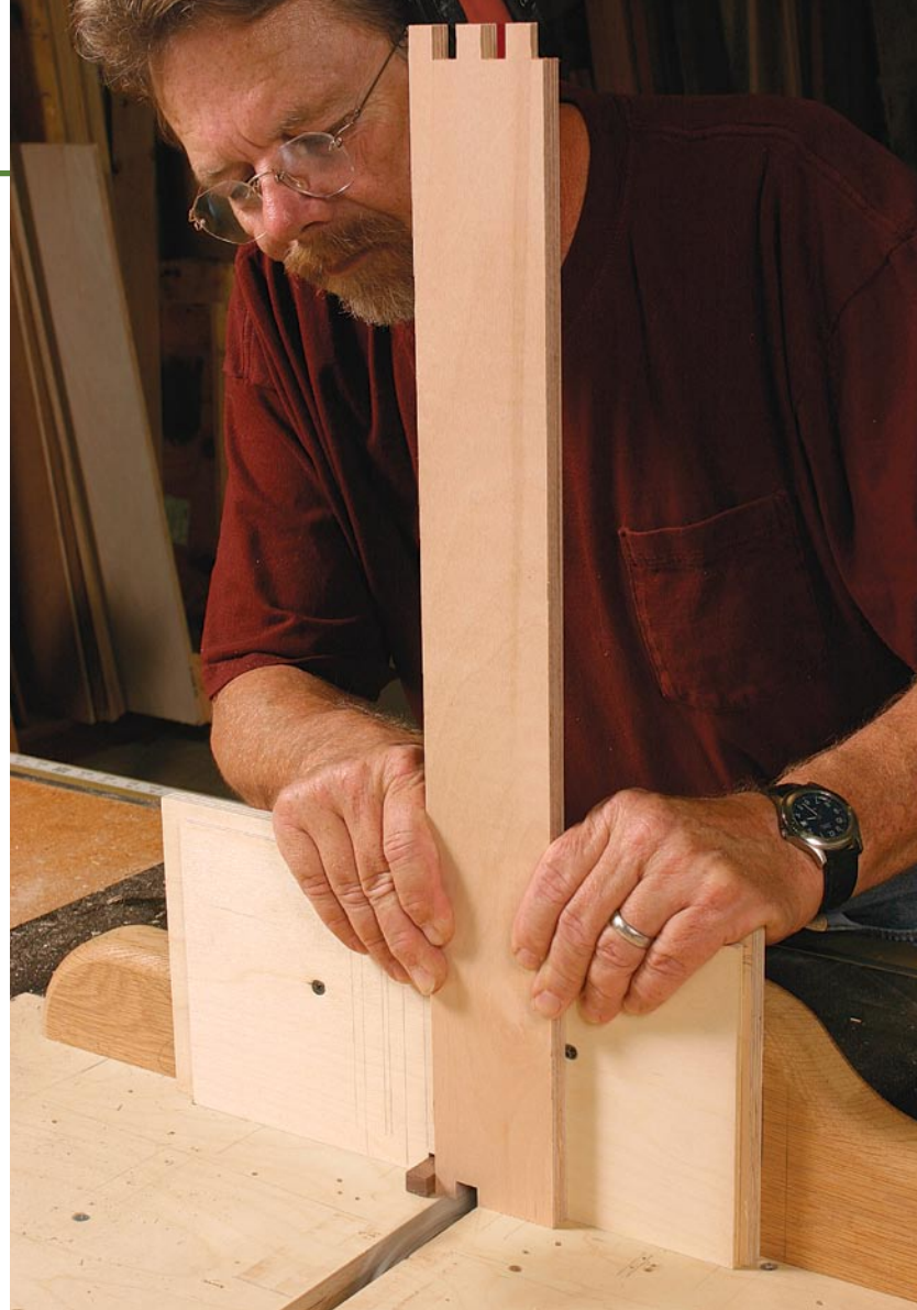
The ends of each piece are identical. For the first cut, butt the top edge of the workpiece against the key.
