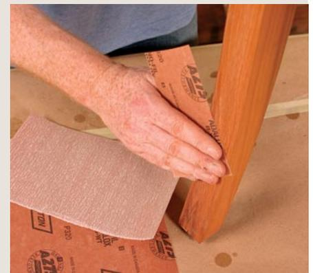
**Smooth the surface.** Between coats of epoxy and before applying the varnish, lightly sand the surface with P320-grit sandpaper.
