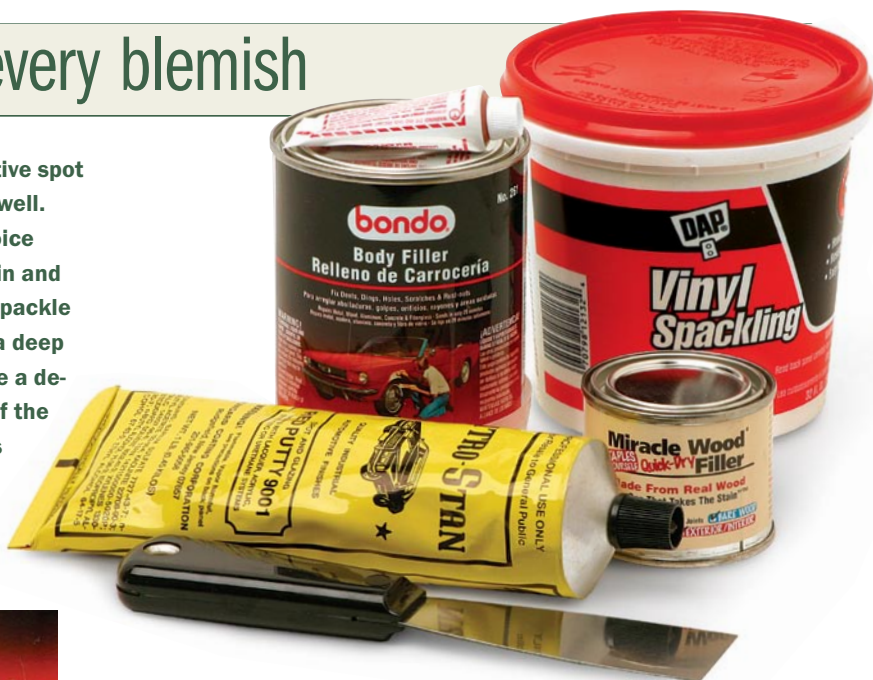
A smooth surface. Large holes are best filled with an auto-body filler that must be mixed with a hardener (far left). Fast-drying wood filler is ideal for medium-size holes (near left).
