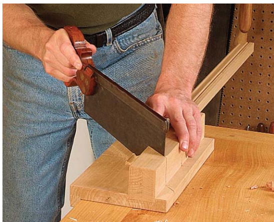
Rough-cut miters. The miter-block bench hook is convenient for cutting small pieces of trim or molding.
