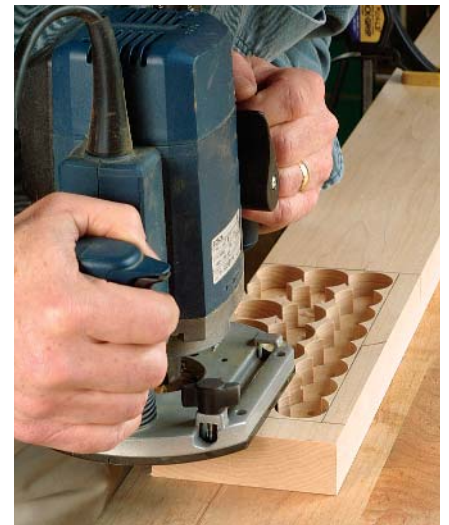
Measure, mark and cut out the mortise. On many vises, the face of the back jaw isn't square to the benchtop. To make sure the mortise ends up deep enough, measure the depth from the thickest part of the jaw. Use a drill bit to remove most of the waste stock before using a router to clean out the waste that remains.
