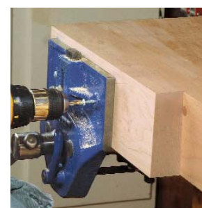
Add the front face. Like the back jaw of the vise, the front jaw is tapered. To minimize the effect of the taper, you can bevel the outside surface of the front face slightly. Then attach the face by driving two screws through predrilled holes in the jaw.
