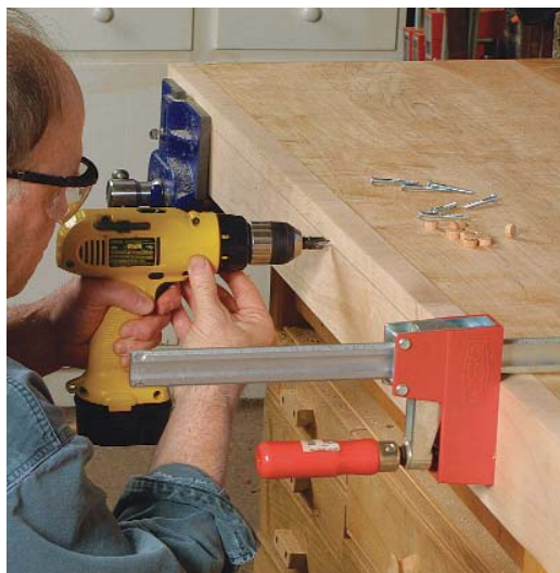
Attach the back face to the edge of the benchtop. To fill in the gap between the back face and the back jaw of the vise, add a couple of strips of epoxy putty to the mortise just before applying the face to the bench (left). After coating the jaw with paste wax, attach the face with a few wood screws driven into counterbored holes (right).
