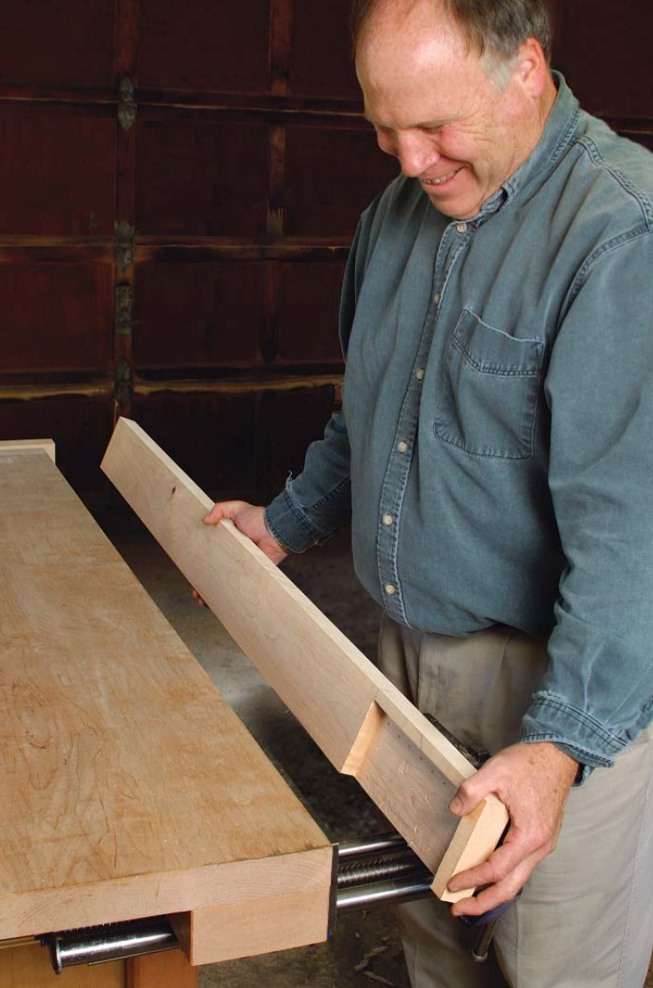
A long face. A mortise in the back face accepts the back jaw. The face extends the full length of the benchtop, which will make it easier to clamp long boards.
