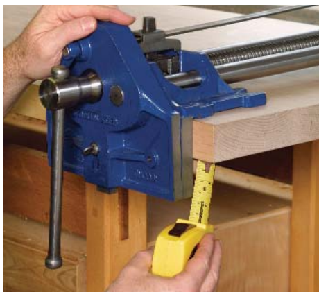
Figure out the filler-block thickness. With both the vise and benchtop upside down to make the job easier, measure the distance from the benchtop to the top edge of the vise jaws and then add \frac{1}{2} in. to \frac{3}{4} in.
