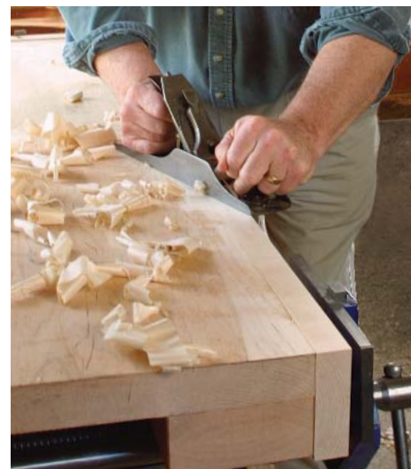
Plane the top edge of the face. A sharp handplane is all it takes to get the face flush with the top of the bench.
