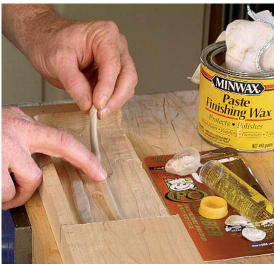
Attach the back face to the edge of the benchtop. To fill in the gap between the back face and the back jaw of the vise, add a couple of strips of epoxy putty to the mortise just before applying the face to the bench (left). After coating the jaw with paste wax, attach the face with a few wood screws driven into counterbored holes (right).
