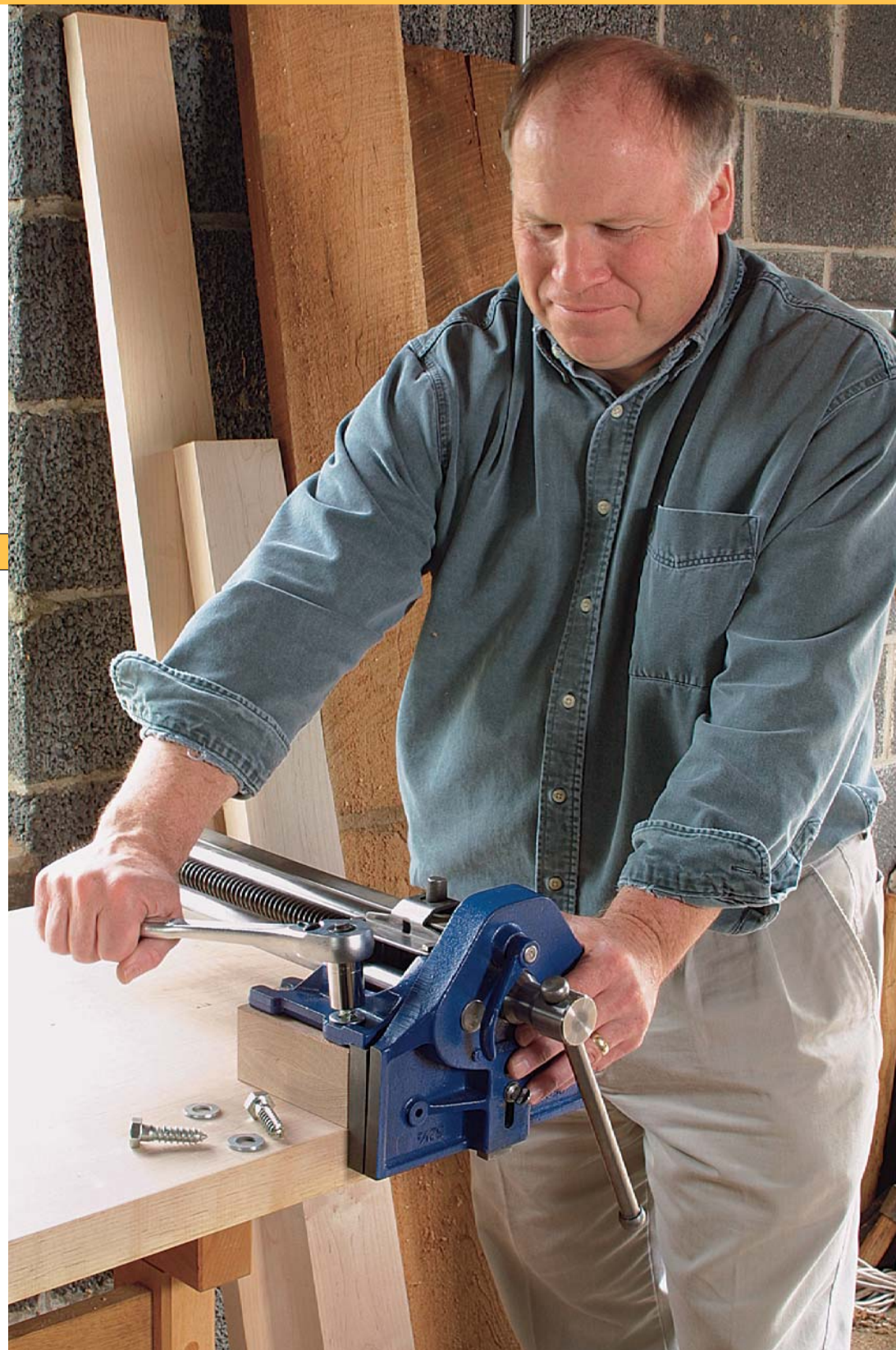
Attach the filler block, then the vise, using lag screws. You might think that about does it, but to get the most out of the vise, you should cover the metal jaws and edge of the table next.
