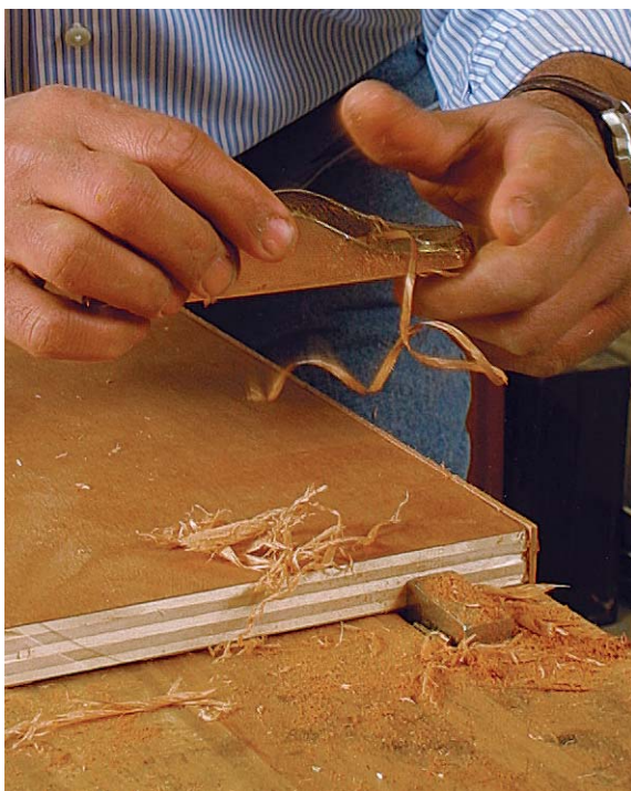
Masking tape makes a good clamp. Numerous short pieces of masking tape provide plenty of pressure for gluing wood edging.
