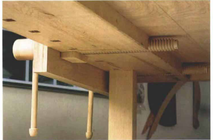
Cut clearance channels for the vise screws. Tap the threaded blocks into place temporarily to determine the location of these channels. Remove the blocks before cutting. Define the edges with a circular saw, kerf out the middle, then chop out the waste.
