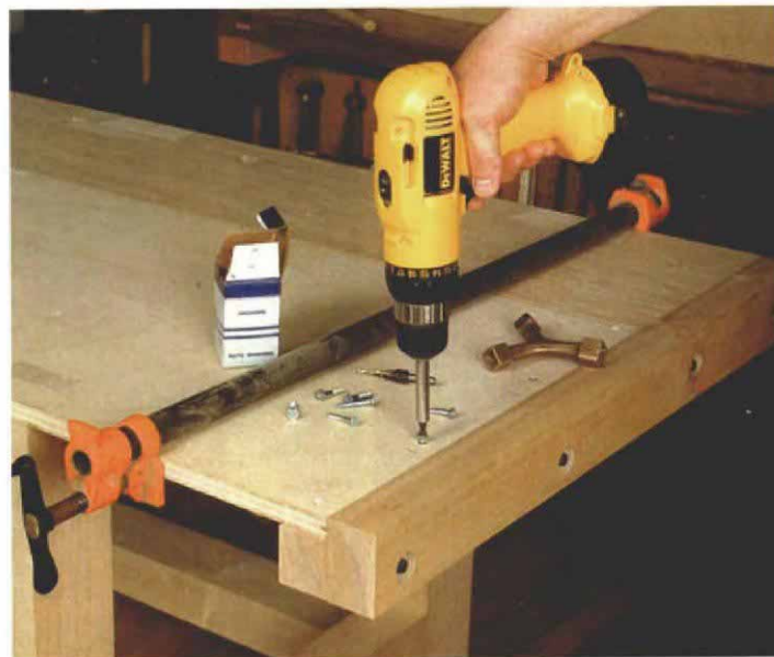
End battens support the plywood portion of the benchtop. Each batten is bolted to the thick plank and also to a cleat that supports the plywood and keeps it level with the plank. The plywood is screwed onto the cleat and into a rabbet at the back edge of the plank.
