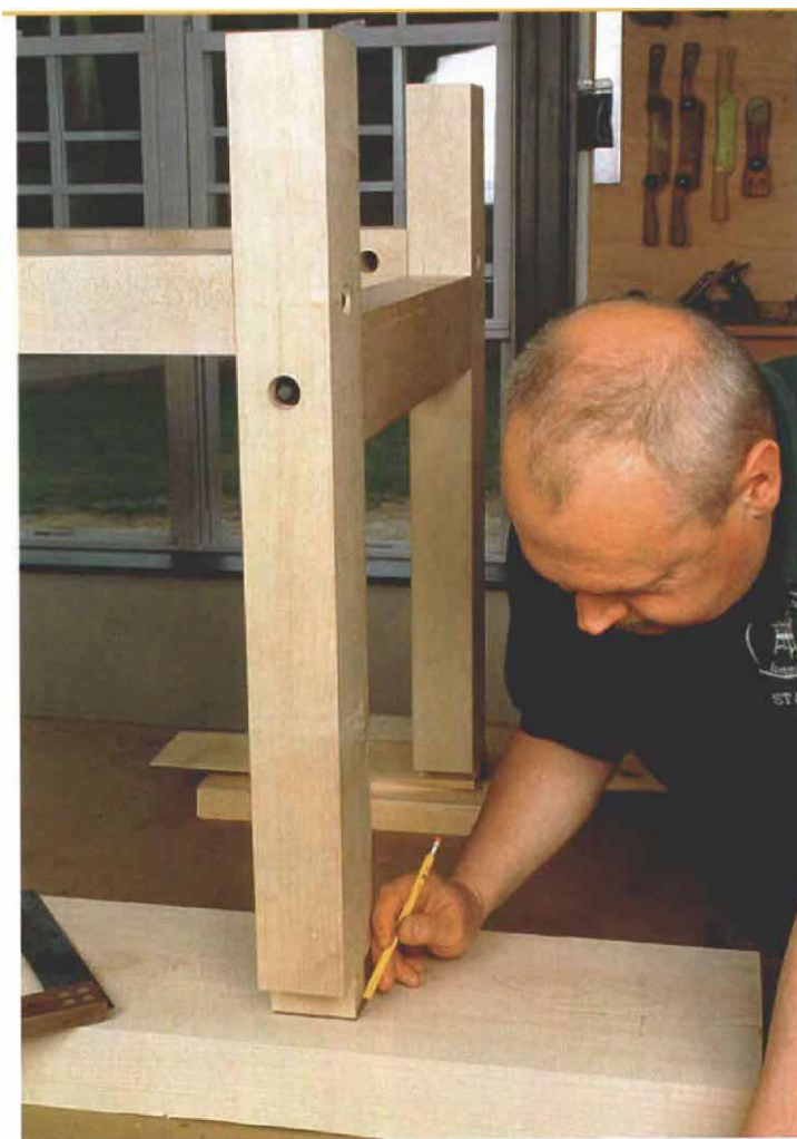
Locate the leg mortises on the plank. First turn everything upside down and level the back legs.
