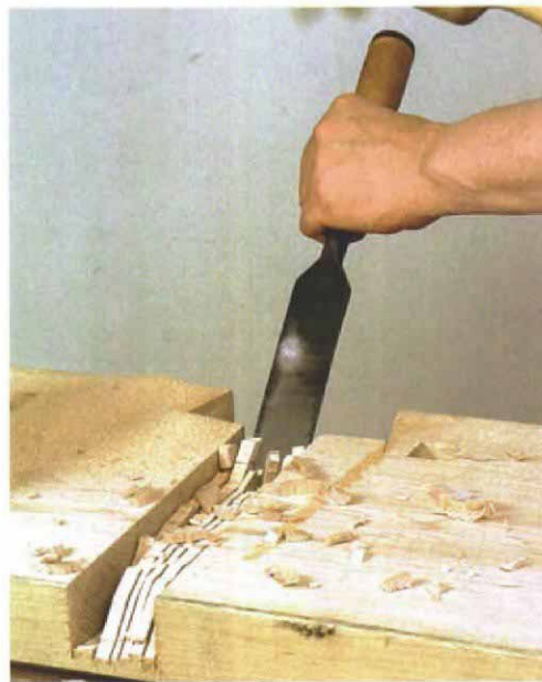
Cut clearance channels for the vise screws. Tap the threaded blocks into place temporarily to determine the location of these channels. Remove the blocks before cutting. Define the edges with a circular saw, kerf out the middle, then chop out the waste.
