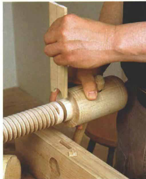
A garter keeps the vise jaw moving with the screw. This thin strip is mortised into the jaw and fits into a groove near the screw hub.
