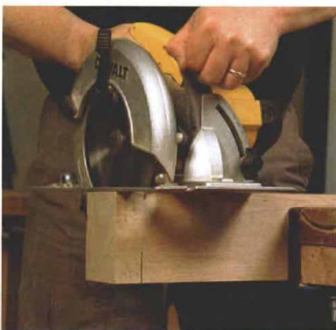
Timber-frame techniques. Use a circular saw to cut the tenon shoulders on these large beams. The cheeks are then cut on the bandsaw. Get an assistant, if you can find one, to help you support the long, heavy timbers. For the mortises in the legs, first drill out the waste, then square with a chisel. Afterward, the tenons are pared to fit the mortises.
