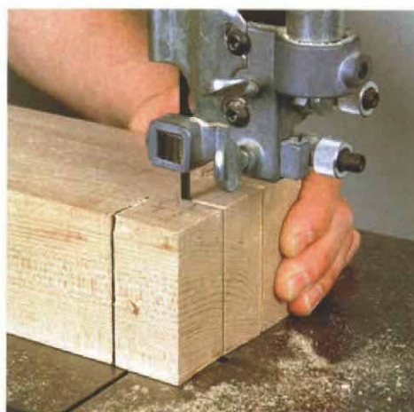
Timber-frame techniques. Use a circular saw to cut the tenon shoulders on these large beams. The cheeks are then cut on the bandsaw. Get an assistant, if you can find one, to help you support the long, heavy timbers. For the mortises in the legs, first drill out the waste, then square with a chisel. Afterward, the tenons are pared to fit the mortises.
