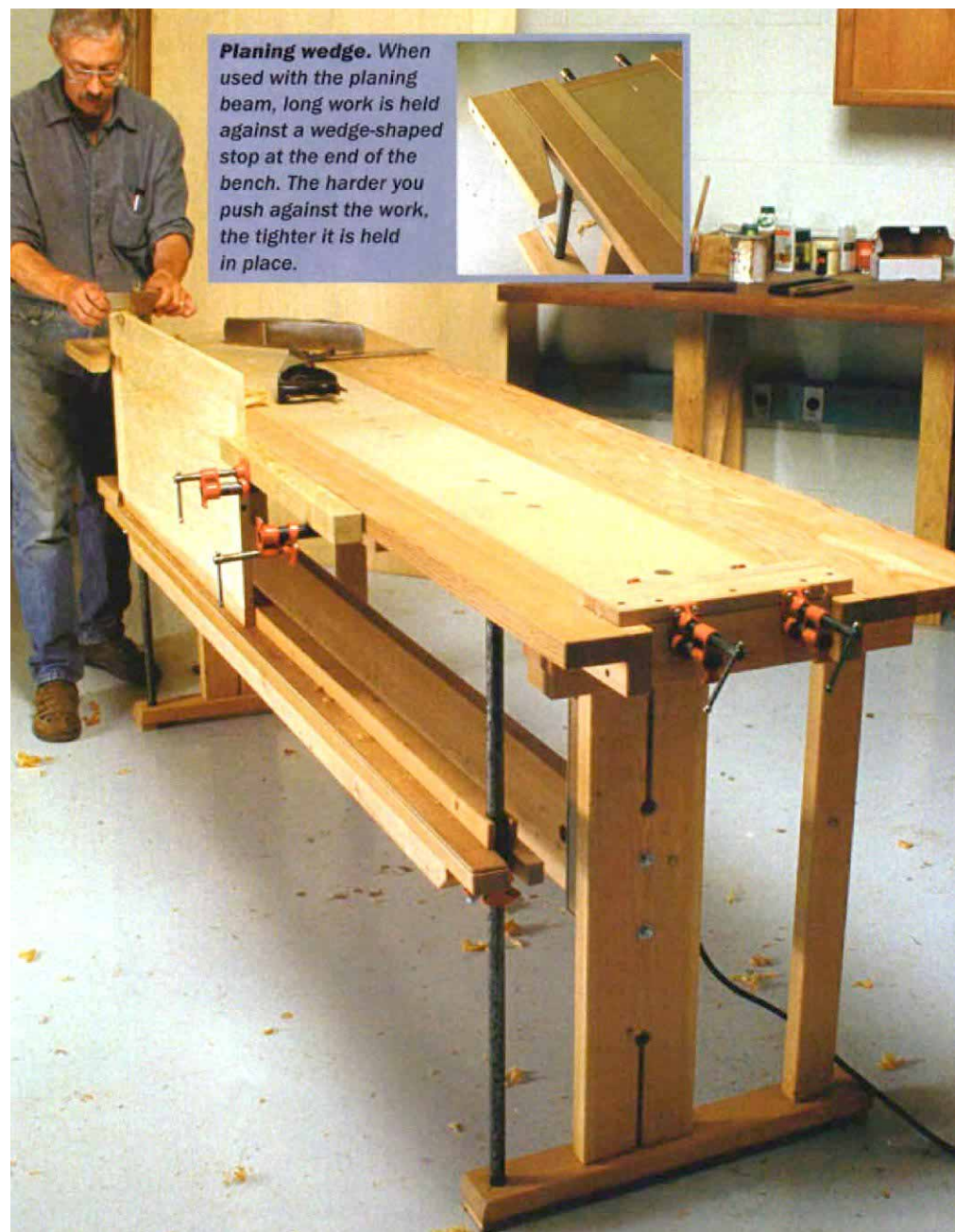
Sliding height adjustment. Pipe-clamp tailpieces slide on cast-iron pipes held captive in the top and bottom of the bench. A T-shaped Douglas fir planing beam rides on the clamps.
