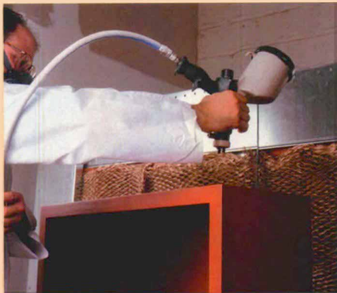
6 Spray the top. By leaving the top for last, the most visible part of the case isn't marred by overspray.
