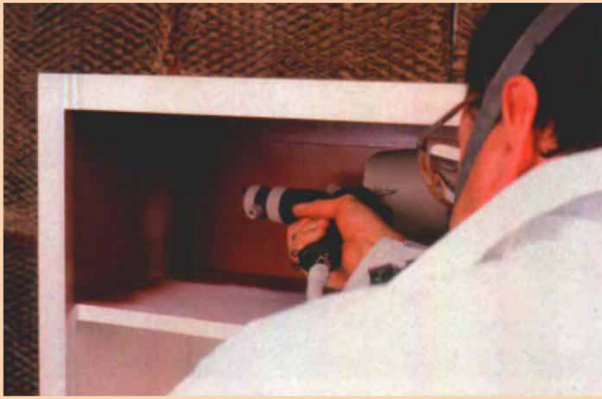
2 Coat interior back and sides. These areas won't be highly visible when the piece is finished.
