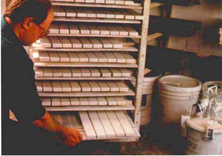
Plan for drying —The author uses racks to cure his spray-finished items. The area is warm, dry and dust-free.
