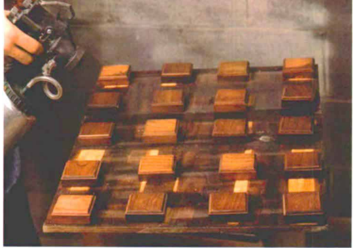
Turntable for even, quick coats —After arranging trophy bases on a lazy Susan, the author sprays with an HVLP gun.
