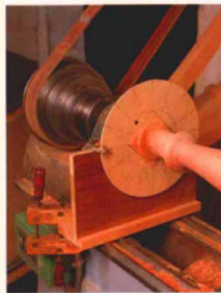
Accurate indexing for reeding. A disc of 1/4-in. plywood makes an indexing wheel for laying out reeding on the bedposts. The stop is a piece of bandsaw blade mounted even with the lathe center.
