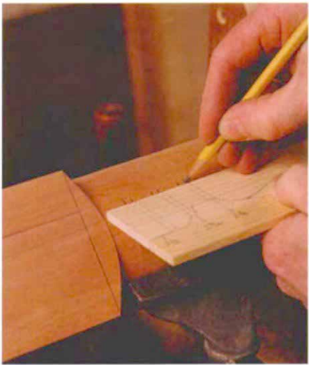
Use a story stick to lay out accurate and consistent turning details. And the story stick is a handy reference when turning because the shape and diameter of each post section is drawn right on it.
