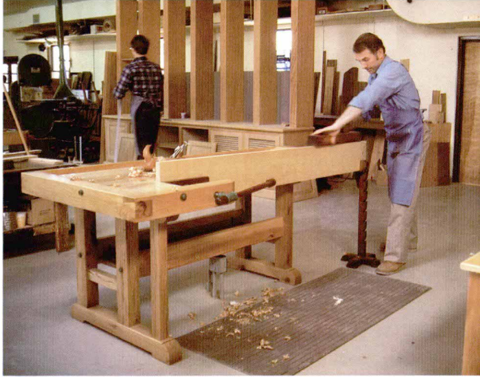
Assemble the 27-in. high utility table with mortise-and-tenon joints. Locate shelves to fit standard plastic drawers for small tools and odds and ends. Larger tools go on the bottom shelf. Make the 40-in. by 60-in. top from particleboard and 1/4-in. maple plywood. To plane long boards, right, Klausz uses a bench slave with the shoulder vise.
