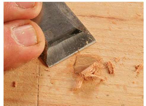
LARGE HOLES Square pegs in round holes. After cleaning up small holes with a Forstner bit, cut a peg slightly larger than the hole. Taper two opposite sides of the peg, round its corners (left), and tap it into the hole (center). When the glue has dried, trim the plug flush (right).
