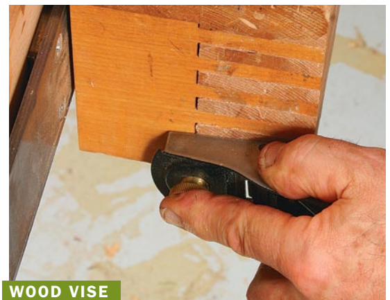
On the level. If joints have become proud (above), plane them smooth so that the two faces of the vise can meet seamlessly. Plane the top of the vise flush with that of the benchtop (right).
