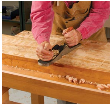
Pick a number. To flatten the benchtop, you can use (from left) a No. 5 plane (bevel up or bevel down), a No. 6, or a No. 7. The plane's length should nearly equal the width of the benchtop (excluding any tool tray).
