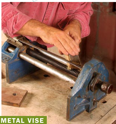
Clean and fresh. To prevent sticking, clean and lubricate the guide bars and the threaded rod (above). Attach fresh hardwood cheeks to the jaws (right).
