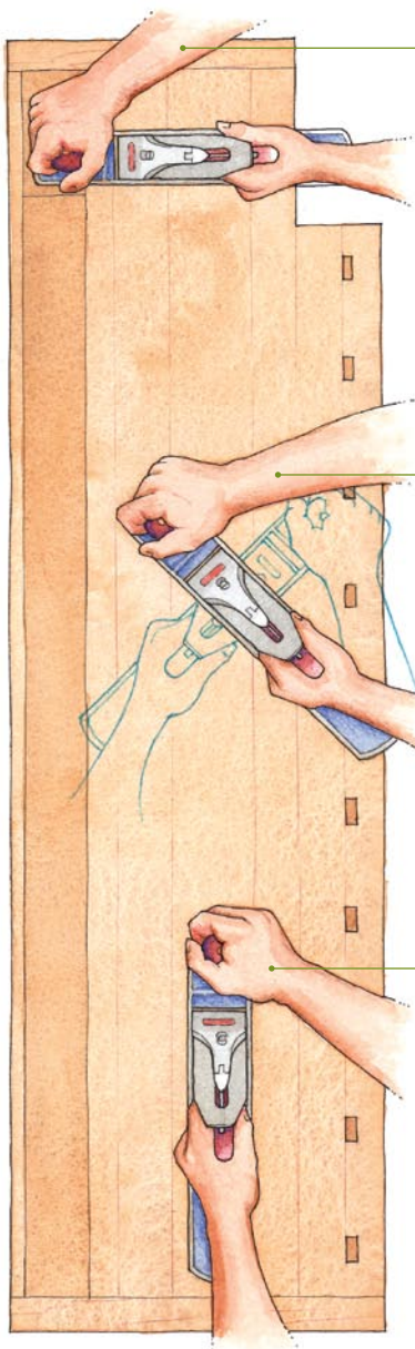
Bevel the edge. To prevent tearout when handplaning across the benchtop, use a block plane to create a small chamfer along the back edge.
