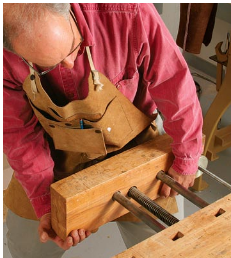
Remove the vises. You'll tune up the vises after the top has been flattened. If your bench has them, unbolt the stabilizing battens (above) and clean out any sawdust that has worked its way down between them and the benchtop.
