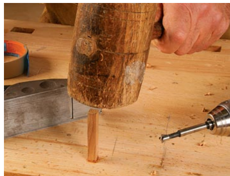
LARGE HOLES Square pegs in round holes. After cleaning up small holes with a Forstner bit, cut a peg slightly larger than the hole. Taper two opposite sides of the peg, round its corners (left), and tap it into the hole (center). When the glue has dried, trim the plug flush (right).
