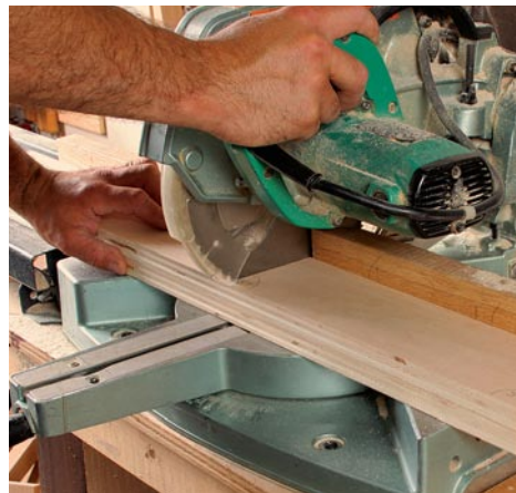
Angle the legs and side pieces. Cut a 5° bevel on the ends of the legs and a 5° angle on the ends of the short stretchers.
