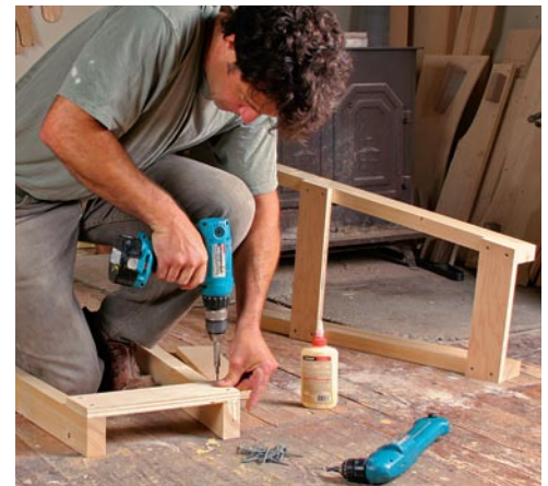
Two drills speed assembly. Start with the short stretchers and legs. Use the first to predrill with a countersink, the second to drive screws.
