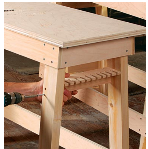
Add the top and a clamp rack. The broad top supports the beams but also adds a handy work surface to the shop. The built-in rack keeps clamps close at hand.
