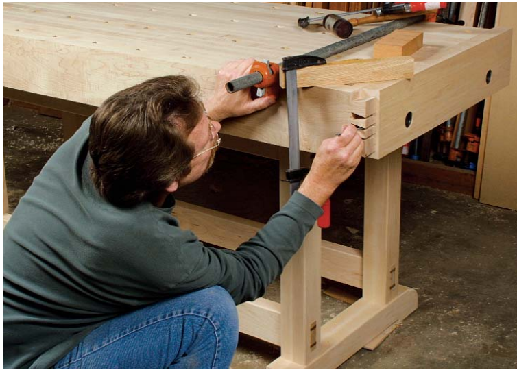
Cut the right-hand set of half-blind dovetails. First, cut the tails in the front apron, and then clamp the front apron in place with the right-hand end cap behind it to transfer the layout of the dovetails.
