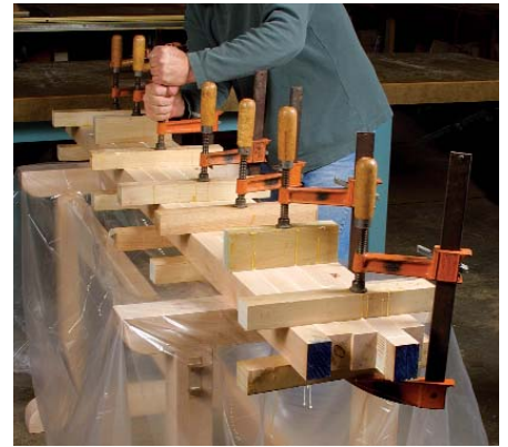
Use cauls to keep the slab flat. Wrap them with clear tape for easy cleanup. Snug them down first, then clamp across the width.
