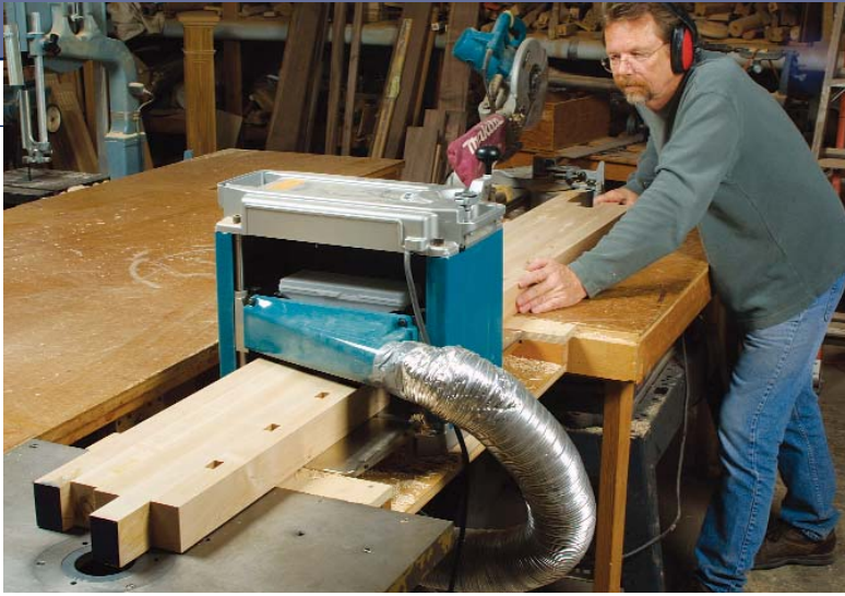
Flatten the slab. A five-board section of the top slab is narrow enough to fit through a benchtop planer.
