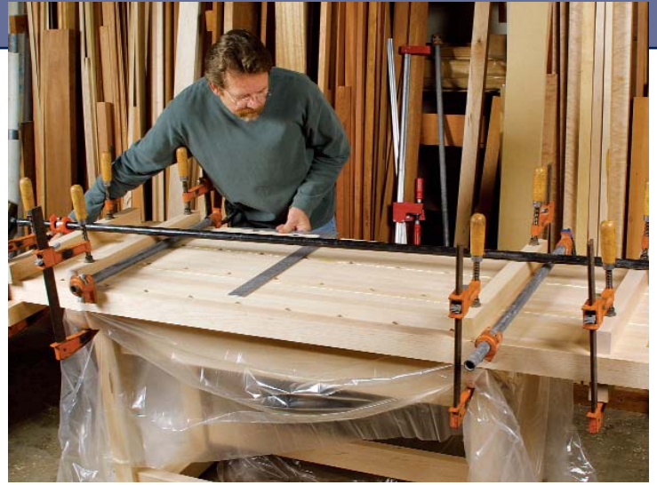
Now glue three sections into one big slab. Place a try square across the dog holes and use a long bar clamp diagonally to correct any misalignment. Again, use lots of clamps and cauls to keep the sections level.
