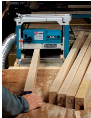
Joint and plane the pieces. Run them through the planer on edge to ensure uniformity.
