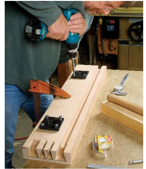
Attach the large vise nuts to the back of the end cap. Also, finish cutting and fitting the dovetails.
