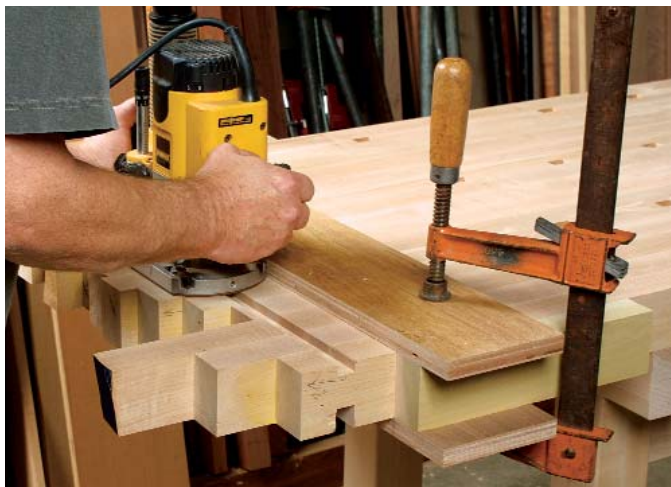
Use the simple two-fence jig shown. Rout deep slots in both sides of the slab, then use a jigsaw to cut off the waste, leaving square shoulders and a tongue that will fit into the end caps.
