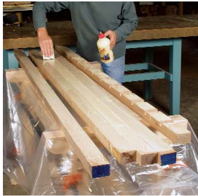
Glue up the top. The base makes a level glue-up platform, but protect it from drips. Use a notched card to spread glue.
