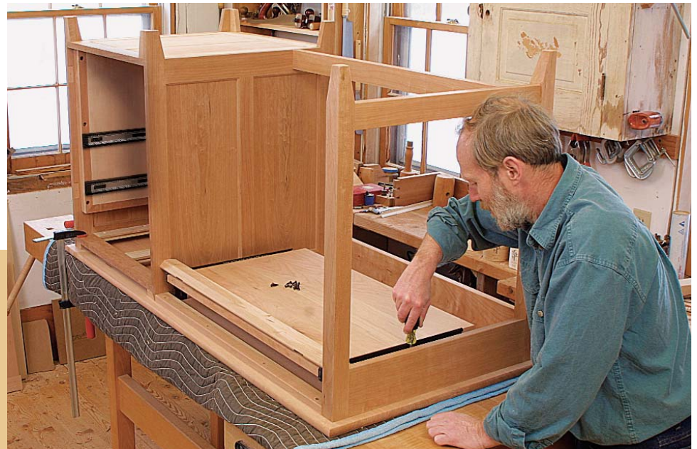
Attach the desktop and the keyboard tray. It is easiest to do this with everything turned upside down. Mount the hardware on the keyboard tray before attaching it to the underside of the desktop.
