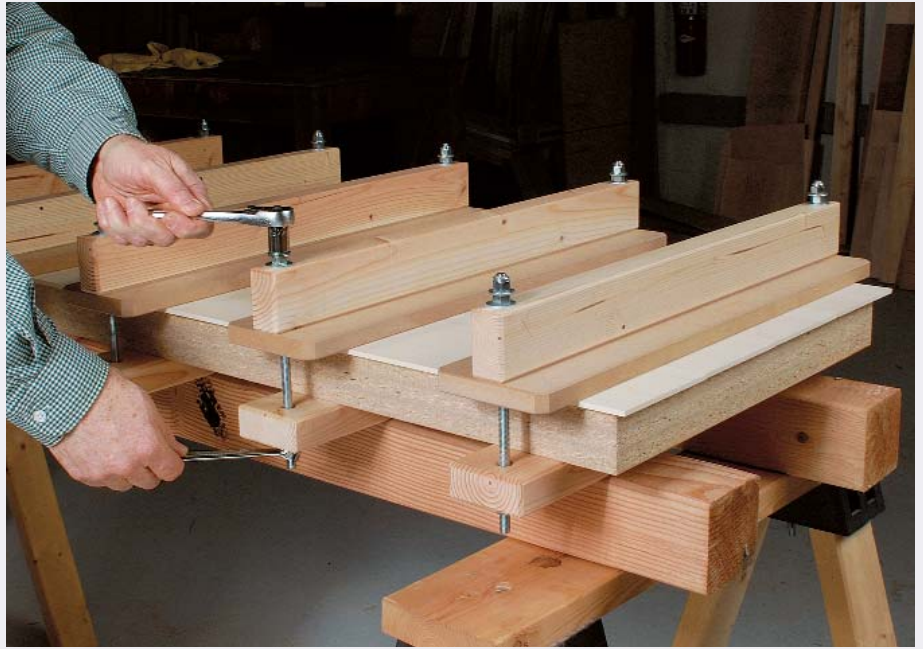
Clamp the veneer to the particleboard with clamping cauls. No need to have a small fortune in clamps to do this glue-up. Shopmade clamping cauls get the job done for pennies.
