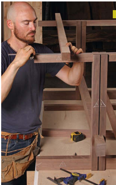
Lay out the joinery for the grid. Dry-assemble the base, mark the locations for all the half laps on the intersecting pieces, and cut them on the table saw.
