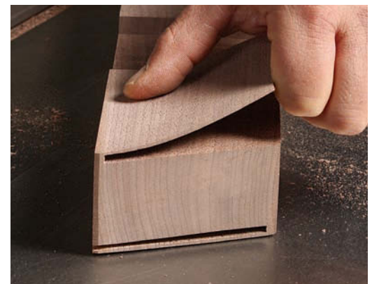
Angle and thin the end of the stretchers. After cutting the angle on each end of the stretcher on the miter saw, use the table saw to trim the block beyond the half lap. With the blade fully raised, rip in and back out (left). Snap off the thin waste (right) and clean up with a block plane.
