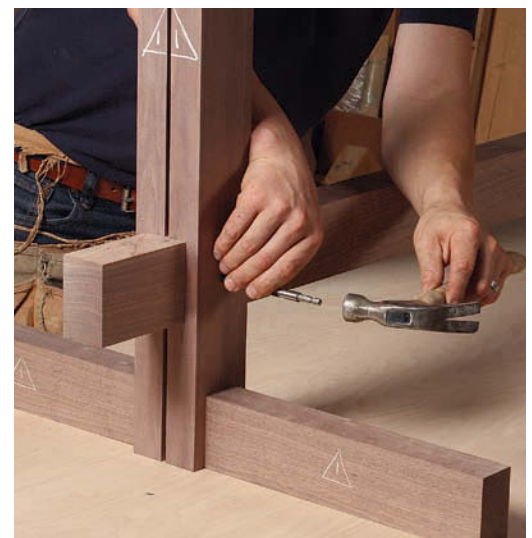
Pegs are a design detail. Locate and drill holes in the posts (left). Dry-fit the feet, stretcher, and posts, and use a brad-point bit to mark the peg location in the stretcher (right). Disassemble and drill the stretcher.
