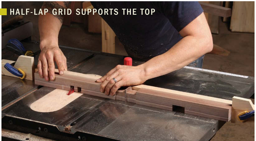
Lay out the joinery for the grid. Dry-assemble the base, mark the locations for all the half laps on the intersecting pieces, and cut them on the table saw.
