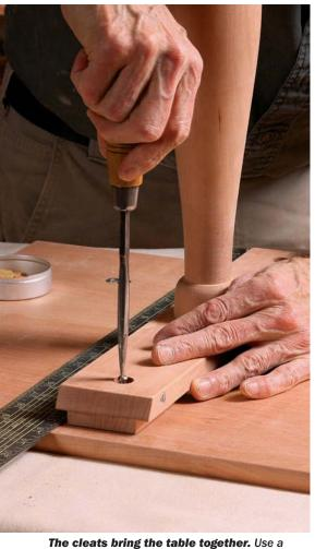
rhe cleats bring the table together. Use a square to align the center cleat on the top, and predrill and screw it in place (above). Then place the drawers against the center cleat. Position the side cleats against the drawer, and attach them (right). A strip of tape on the drawer side gives you a little wiggle space once it's removed.
