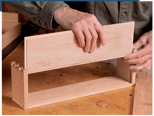
**Two-faced drawers.** Through-dovetails are visible on the fronts and sides of these drawers. Because there are two fronts, a rabbeted drawer bottom gets inserted during the glue-up (above). Use an end-grain plug to fill the exposed drawer bottom grooves on the drawer faces. A simple long-grain to long-grain glue joint is strong enough to attach the runner to the side of the drawer (below).
