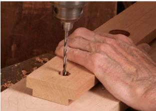
**Drill and attach the center cleat.** Use a Forstner bit to cut a through-mortise for the post in the center cleat (top). Each cleat also gets a hole on each end (above). Elongate the holes with a file to accommodate wood movement. Finally attach the center cleat to the post (right). Glue and wedge the mortise-and-tenon joint, aligning the cleat so it's centered with one of the legs. Then trim it flush.
