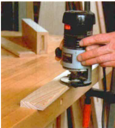
One tenon fits all. The author mills tenon stock to thickness, rips it to width, then rounds over the corners. By trimming them to short lengths, he can make many tenons from one piece of stock.
