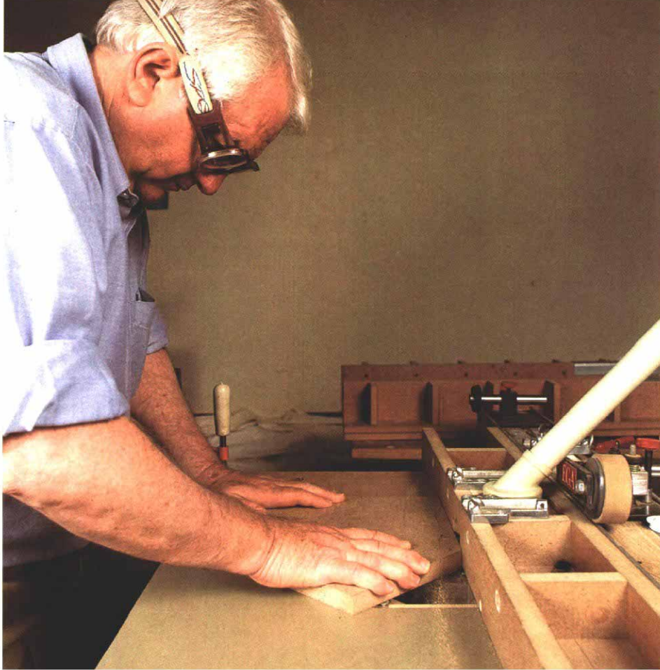
Dealing with dust—A worker in the Sackler Gallery cabinet shop (above) at the Smithsonian Institution avoids the fine dust produced by MDF by wearing a Racor powered respirator while finish-sanding a display cabinet.
