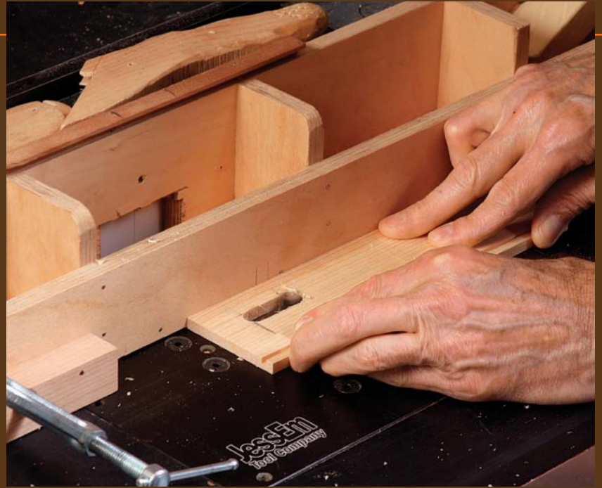
Stopped slot. At the router table, plunge-cut the guide slot in the drawer's long side. Set stop blocks to control the length of the slot, and be certain to anchor the workpiece against a stop block when making the plunge.
