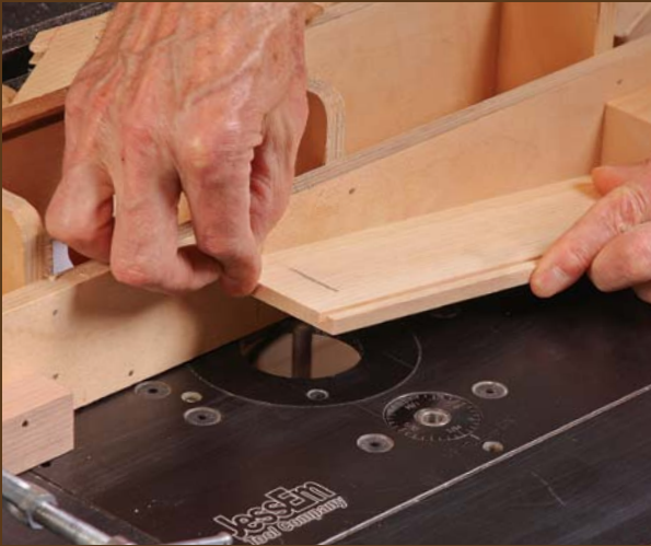
Stopped slot. At the router table, plunge-cut the guide slot in the drawer's long side. Set stop blocks to control the length of the slot, and be certain to anchor the workpiece against a stop block when making the plunge.
