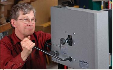
**Quick-release tension speeds up blade changes.** Most saws have a lever that releases or engages tension on the blade. Flip the lever and the tension releases instantly. Without it, blade changes take longer.
