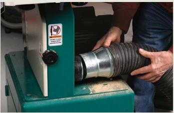
Lower ports miss too much dust. Falling dust is able to escape the port's reach. Both the Grizzly (shown) and Hammer saws have low ports.
