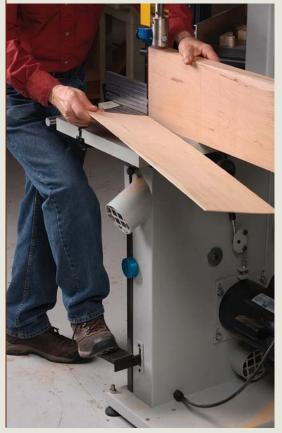
Stop it with a step. The foot-activated brake frees up both hands to control the workpiece. Five saws have a foot brake: General International, Hammer, Laguna 14 SUV (shown), Powermatic. and Rikon 10-351.
