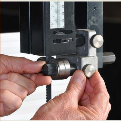
**Tool-free is the way to go.** The guides on the Powermatic PM1500 were the easiest to set up and adjust.
