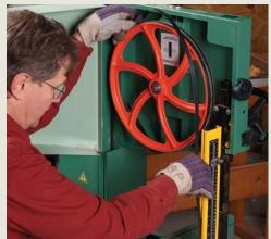
Window makes blade tracking easier. You can see when the blade is centered on the tire. The Hammer, both Laguna machines, and both Rikon saws have one. A light-colored tire, like the one on the Rikon 10-325 (shown), is a great aid, too.
