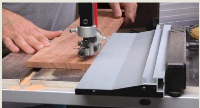
**Two-position fences are safer.** No matter how tall the workpiece is, you can always get the guide bearings close to it with this type of fence. The lower position also provides plenty of clearance for your hand or a push stick.
