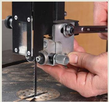
**Tools slow you down.** The guides on the Rikon 10-325 require two different wrenches (one box end, one Allen), making adjustments more cumbersome.
