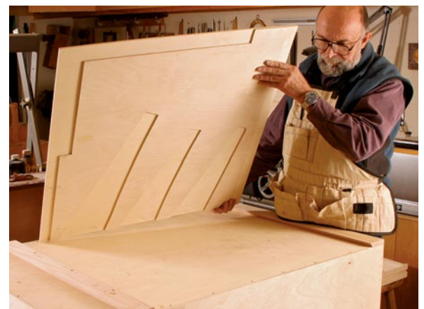
Storage behind the cabinet. An inner layer of \frac{1}{4} -in.-thick plywood is cut to receive panel saws and a carpenter's square, then covered by a solid outer piece of plywood.
