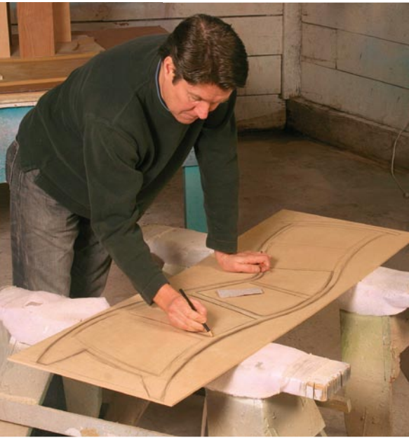
Refine the design at full size. Beaumont draws on ¼-in.-thick MDF, using sandpaper as an eraser and working the drawing until it pleases his eye.
