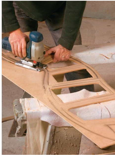
Cut the template with a jigsaw. He drills a hole in each corner of the drawer openings and then saws between them to remove the waste.
