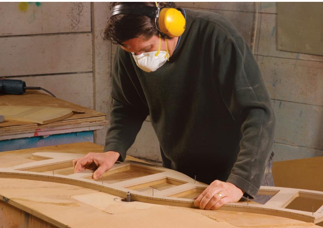
Rout the front flush. After smoothing all the edges of the template, inside and out, Beaumont uses it to rout the front (and back) of the cabinet using nails to hold them together temporarily.
