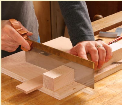
Mark and cut. For the sides of this jewelry tray, Kenney measured directly from the workpiece (left), then cut the parts at the saw hook (right). Generally, it's best to leave the pieces a little long and then square the ends and fine-tune the fit at the shooting board (see next page).
