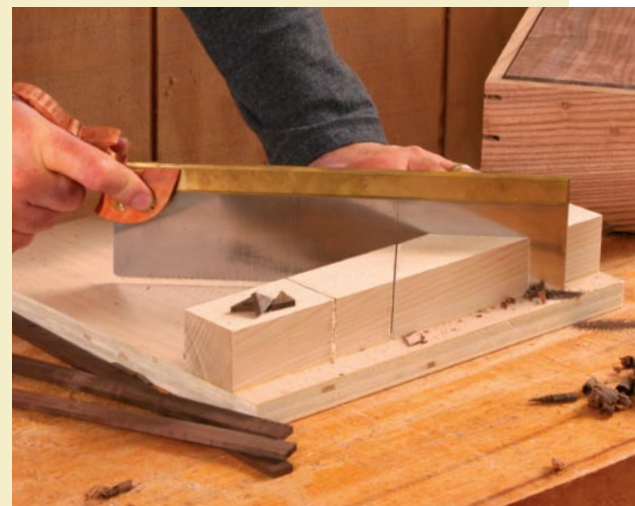
45° too. The same goes for miters. Here, Kenney trims the waste off the corner keys he planed on the previous page.
