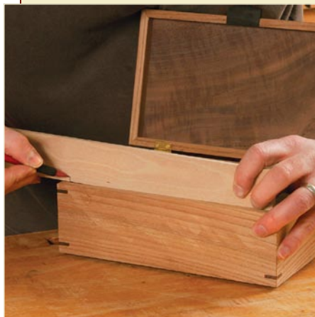
Mark and cut. For the sides of this jewelry tray, Kenney measured directly from the workpiece (left), then cut the parts at the saw hook (right). Generally, it's best to leave the pieces a little long and then square the ends and fine-tune the fit at the shooting board (see next page).
