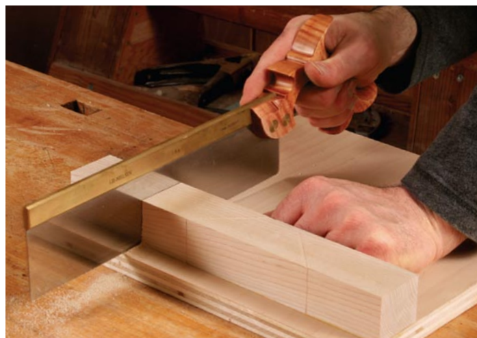
Fence gets three cuts. After attaching the fence and hook, lay out the 90° and 45° cuts in the fence with a marking knife and square (left). Then make a shallow groove with a chisel (center) to guide the backsaw. Cut the kerfs with the same saw you'll use to cut stock (right).
