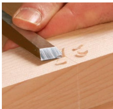
Fence gets three cuts. After attaching the fence and hook, lay out the 90° and 45° cuts in the fence with a marking knife and square (left). Then make a shallow groove with a chisel (center) to guide the backsaw. Cut the kerfs with the same saw you'll use to cut stock (right).
