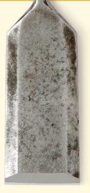
Fix the nicks first. There's no point in honing this edge until the nicks have been removed. Puchalski uses a block of wood to hold the chisel perpendicular to the sandpaper as he grinds the edge back to remove the nicks. Then he regrinds the primary bevel with the chisel in a honing guide. The same method works for plane blades.
