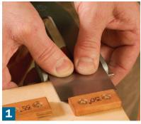
This should take only a minute. Use the 30° stop on the board to set the iron in the honing guide (1). Four or five passes on the 1,000-grit stone should be enough to raise a burr on the iron's back (2). Take a handful of passes on the 8,000-grit stone to create a highly polished narrow band at the tip (3). Finally, repeat the ruler trick to remove any remaining burr on the back (4).
