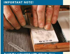
Avoid the ruler trick with chisels. Once you're done honing, take a couple of passes on the back to remove the burr. Keep the back flat on the stone.
