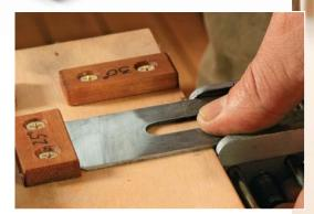
Set the angle. Most primary bevels are ground at or near 25°. Puchalski uses sandpaper in grits ranging from P80 to P400. He attaches the paper to a flat slab of granite and repeatedly works through the grits, taking about 10 to 15 passes over each grit.
