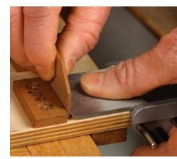
Shim adjusts angles. The 1/8-in.-thick shim adds about 2° to shallower angles and up to 5° to steeper ones.
