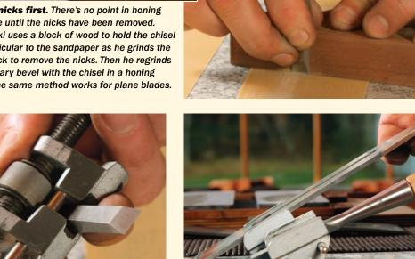
The angles are different. Chisels ride lower in the honing guide and project farther out of it. To compensate, choose a stop that is 5° steeper than your desired angle.
