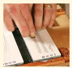
Honing in two steps. Puchalski works the entire face of the bevel on the 1,000-grit stone, then hones a secondary bevel a few degrees steeper on the 8,000-grit stone.
