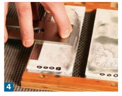
easily on the 8,000-grit stone by placing extra pressure on the narrower side with just a few more strokes. As a final step, remove the blade from the honing guide and touch up the back using the ruler trick to fully remove any burr that is still present.
