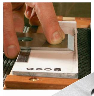
It's more efficient to create a small, steeper secondary bevel right at the cutting edge. For the most common primary bevel of 25°, a secondary bevel of 30° works well.
