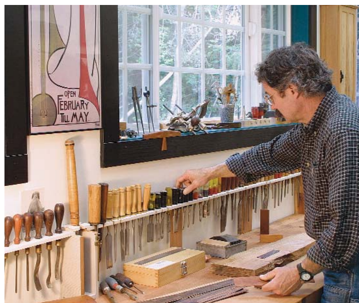
Cutting tools in line. On his other bench (across from the planes), Van Ornum keeps his chisels and carving gouges within easy reach.
