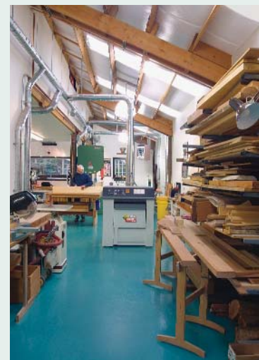
Efficient layout. Machines are arranged so that wood progresses in logical order from the lumber rack through all of the workstations.
