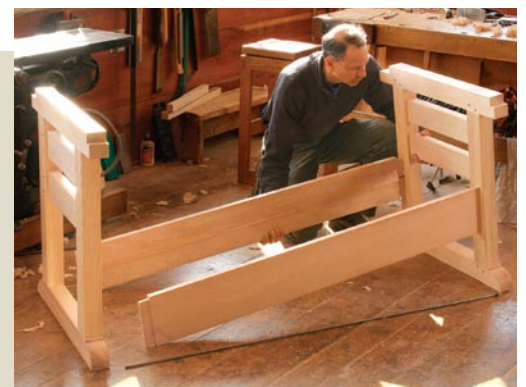
Big stretchers. Threaded rod gives a secure connection between the stretchers and trestles.
