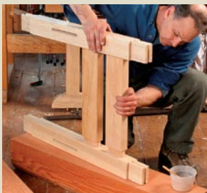
Wedge the shoes. The mortise-and-tenons in the top and bottom of the trestles are wedged.
