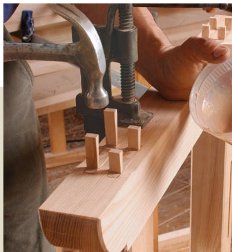
Wedge the shoes. The mortise-and-tenons in the top and bottom of the trestles are wedged.
