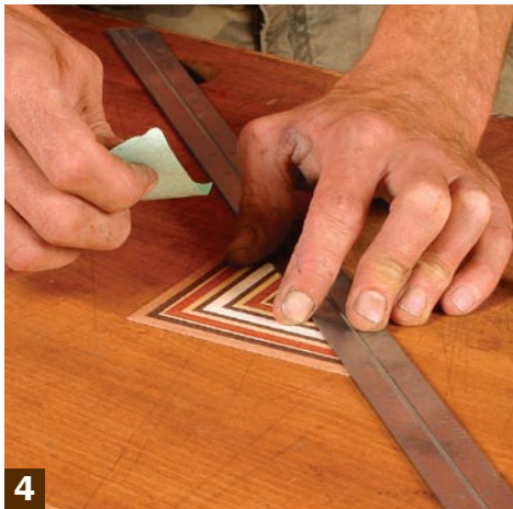
4 Begin assembling the puzzle. Use a straight-edge to align a pair of shapes and tape them together on their rougher, bandsawn faces.
