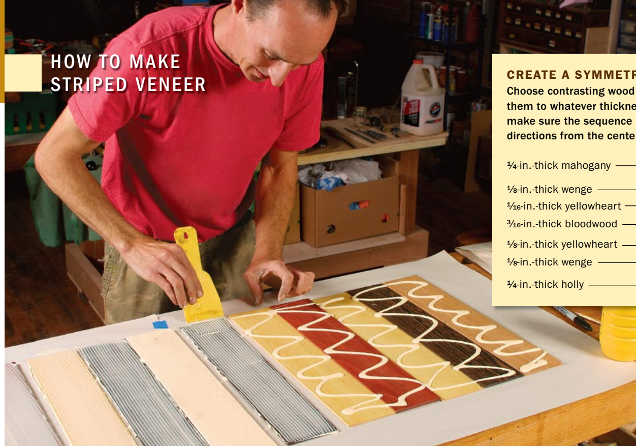
Glue the contrasting woods. Ferrazzutti uses a notched spreader to apply a liberal amount of yellow glue to the strips of colored woods.
