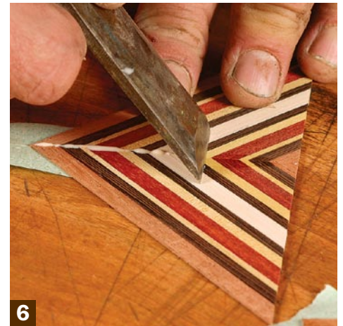
6 Close the joint. Use the back of a chisel to remove squeeze-out and bring the joint flush. Tape this face side while the glue dries.
