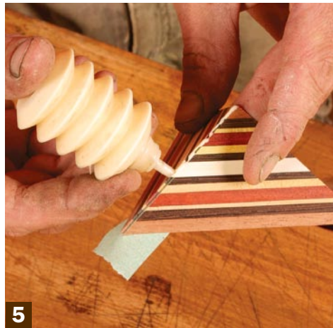
5 The hinge trick. Flip over the pair of pieces, open up the joint using the tape as a hinge, and apply a thin bead of glue.
