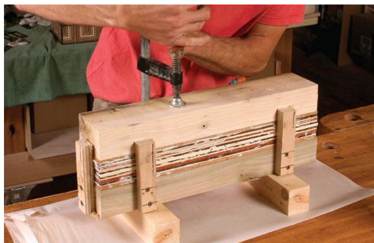
Glue the contrasting woods. Ferrazzutti uses a notched spreader to apply a liberal amount of yellow glue to the strips of colored woods.
