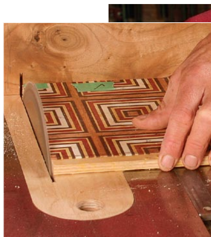
Add the top and bottom. When cutting these pieces to fit into their rabbets, make sure that the veneer pattern is aligned. Then glue and clamp them into place.
