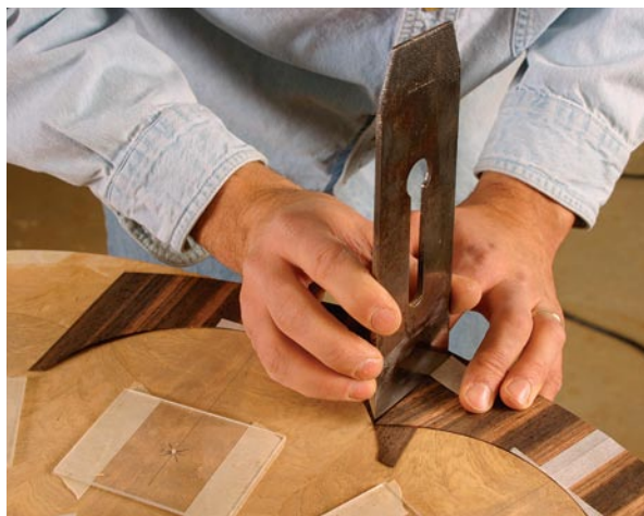
Align the pieces. Place the book-matched joint in the border on the center line of a sunburst segment. Then cut the veneer along a line that extends from the sunburst seam.
