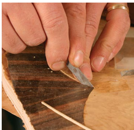
Cut the corners. A knife extends the groove into the corners where adjacent arcs meet.
