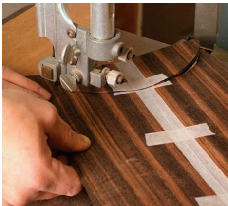
Profile the border. Book-match the veneer and then bandsaw the concave profile in a stack.
