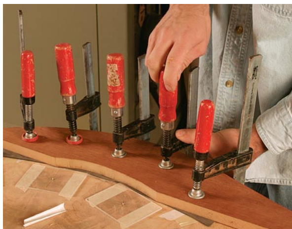
Glue one or two sections at a time. Place a bit of plastic film followed by a piece of rubber sheeting on top of the sections. The rubber allows uneven thicknesses of veneer to receive even pressure while the plastic prevents the rubber from getting glued to the veneer.
