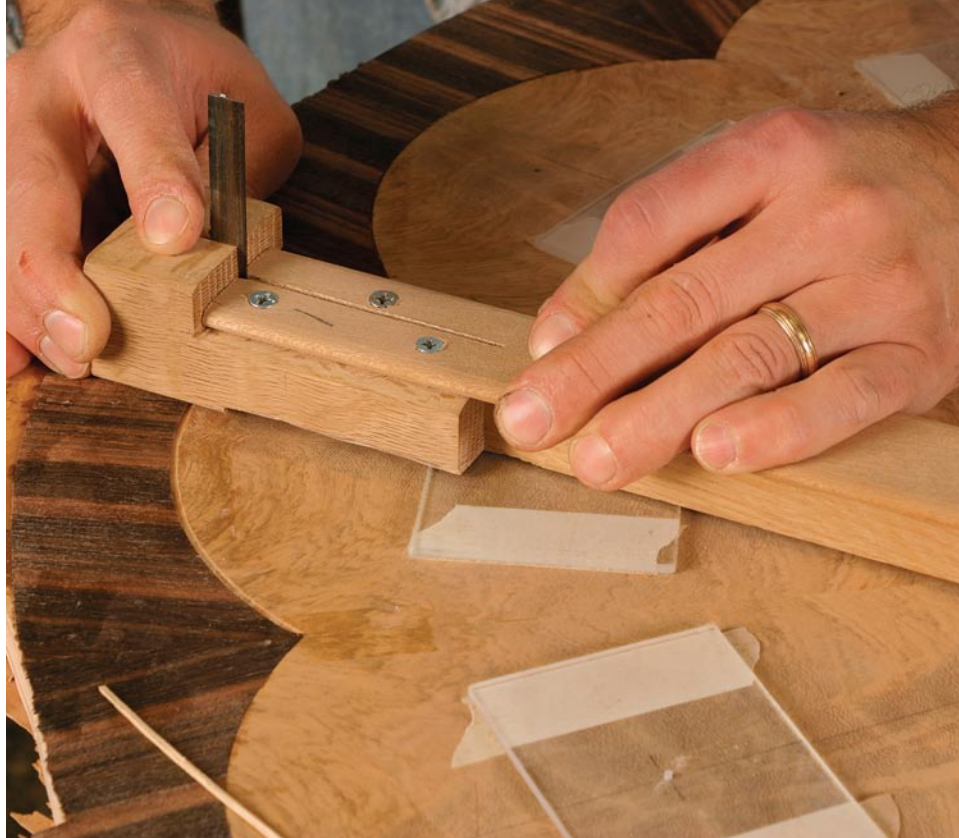
Same pivot point. Use a scratch stock on a trammel to cut a groove between the sunburst and the border veneers.
