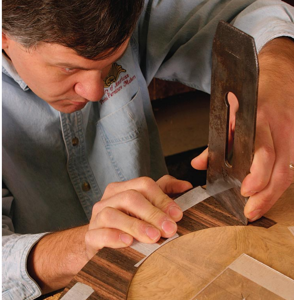
Align the pieces. Place the book-matched joint in the border on the center line of a sunburst segment. Then cut the veneer along a line that extends from the sunburst seam.
