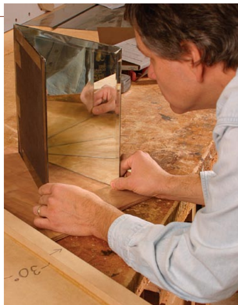
Look in the mirror. Two mirrors angled at 30° preview what the finished sunburst will look like.
