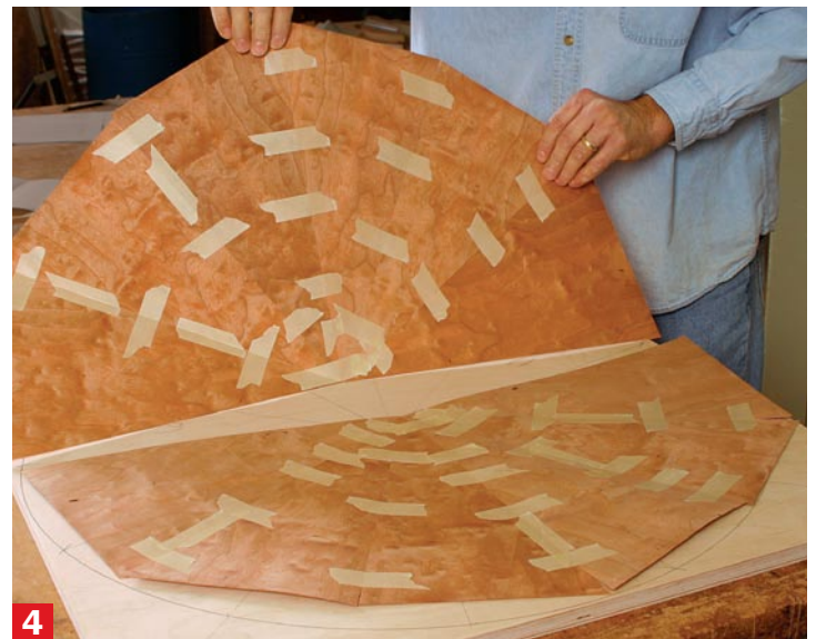
4 Two halves completed. Join adjacent quarters to form two halves that extend about 190°.
