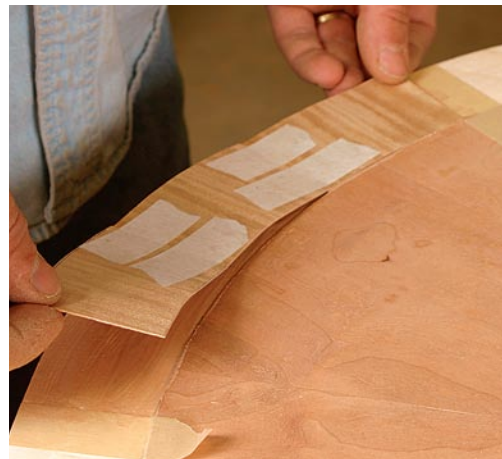
Three at a time. Tape three pieces of veneer together, lay them on the substrate, and place masking tape at both ends to help remove glue squeeze-out.
