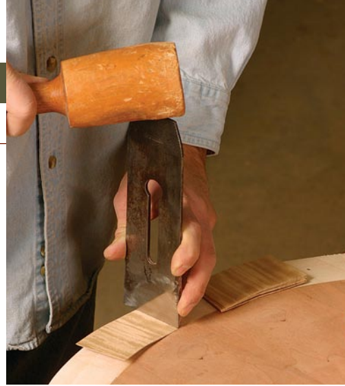
A clean cut. A plane iron creates a tight seam when joining the sections.
