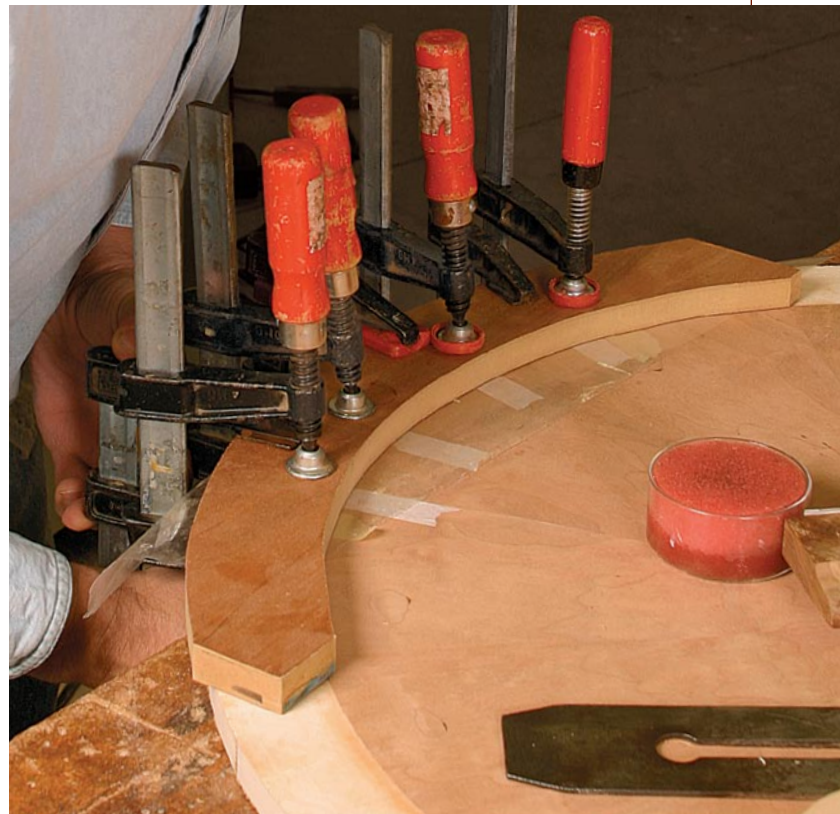
Clamp with a curved caul. After applying glue to the substrate, tape the border to the sunburst to prevent it from moving when clamping pressure is applied.
