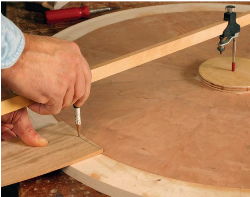
Prepare the sections. Use a trammel to scribe the sunburst curve onto a stack of border veneer.
