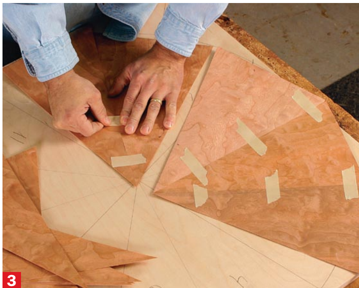
3 Quarter by quarter. Beginning with an oversize segment, use masking tape to assemble each quarter, flipping and book-matching alternate segments.
