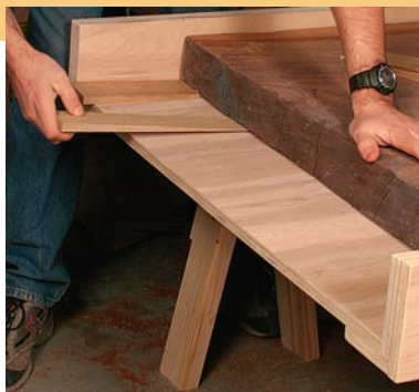
Steady the slab. Push shims under the slab to prevent it from wobbling in the jig as you flatten the face.
