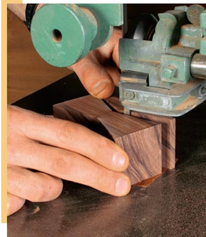
Cut the key on the bandsaw. Use a disk sander to smooth the cut edges, keeping the sides flat and square.
