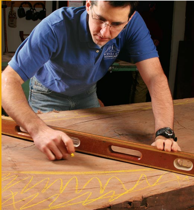
Mark the high spots. Lay a long straightedge across the slab to find its high spots, then mark those areas with a pencil or a lumber crayon.
