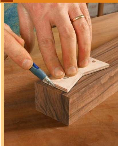
Mark the blank. Trace the shape of the key onto the blank, with the grain oriented lengthwise.
