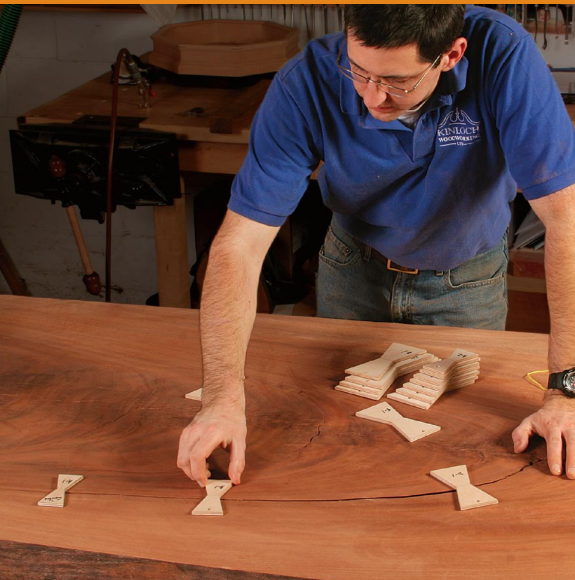
Lay out the keys. Well-placed butterfly keys stabilize or hide defects, and enhance the handcrafted, organic look. Zuba uses a series of templates to decide how large to make each key and where to position them. Then he marks their location on the slab.
