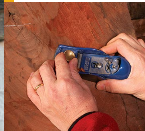
Plane a patch. You can check the wood's color and grain by smoothing a small area with a block plane.
