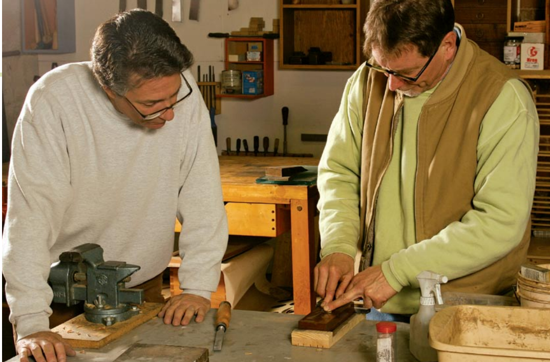
Lock the arms to lock in the angle. Rogowski showed Cecala how to concentrate pressure on the blade's tip while keeping his arms rigid to help maintain the honing angle.
