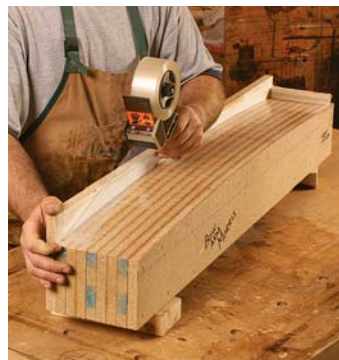
Finish the form. Screw a melamine fence to the rear of the form and a stop to its front edge. Packing tape keeps the glue from sticking to the form and stop.
