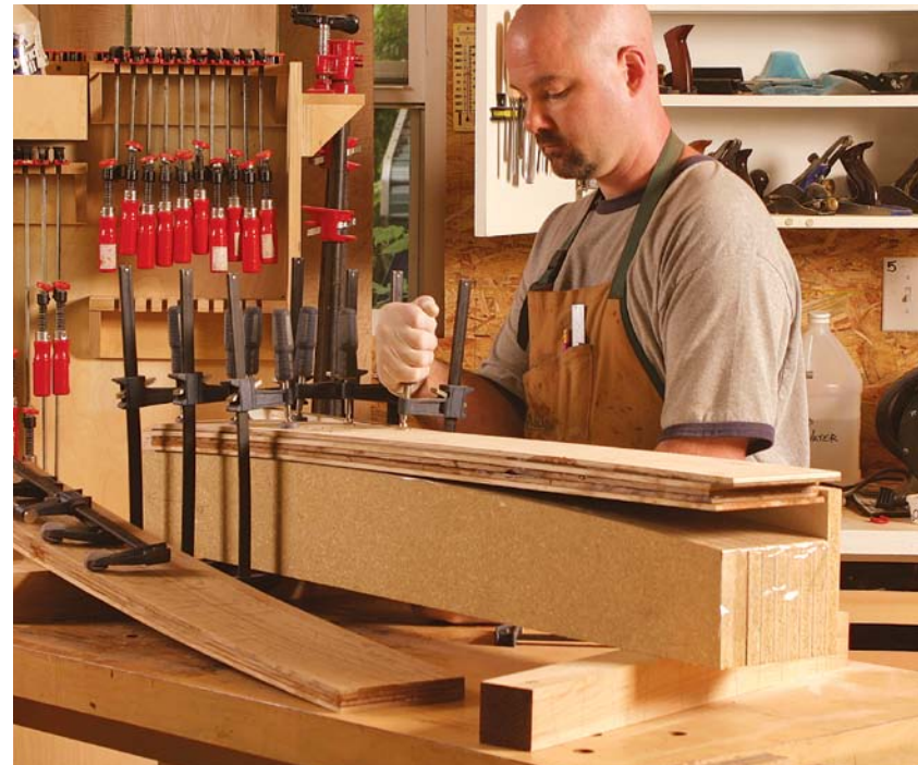
Clamps, clamps, clamps. After coating the plies with glue, press them against the stop and fence. Add a flexible caul on top and start clamping next to the stop. Work progressively down along the form. Place a clamp every 2 in. You'll need two dozen.
