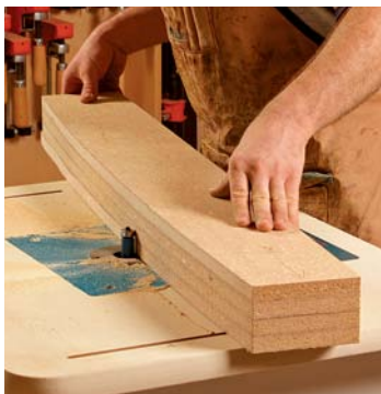
Build the form layer by layer. Make the first layer at the bandsaw, cleaning it up with sandpaper. Glue and screw on each successive layer and rout it flush.
