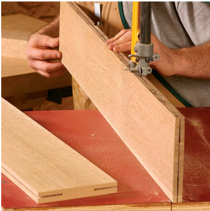
Resaw the plies. Start the cuts on the table saw and use the kerfs to guide the bandsaw blade as you finish the cut freehand.
