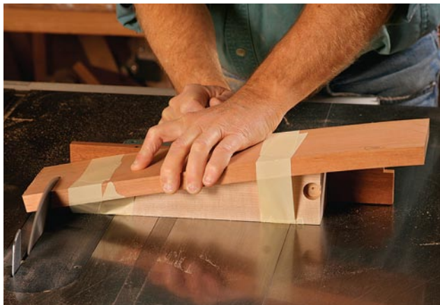
Support block for trimming and tenoning the ends
