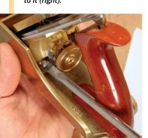
Set the mouth opening. Small screws allow you to adjust the mouth opening to accommodate heavy or light cuts (right).
