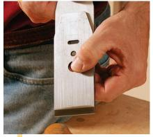
Secure the chipbreaker. Keep its leading edge slightly inset from the front of the blade, and parallel to it (right).
