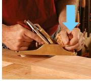
**Power up.** For stability and power, stand with your legs comfortably spread apart and your feet facing forward. Lean slightly forward, and put firm, downward pressure on the knob as you begin the cut.
