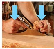
Full contact. Once the plane's sole is completely on the board, apply pressure equally to both the tote and knob. Skewing the plane will reduce resistance and help eliminate chatter. Be sure to maintain your wide stance and use your body to drive the tool forward.
