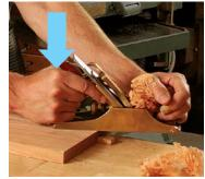
**Exit strategy.** As you exit the board, ease up on the knob and focus pressure more on the tote. Continue working across the board using consistent, overlapping passes.
