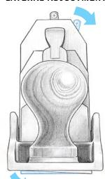
Move the lever toward the heavy side of the cut to bring the shaving to the center.
