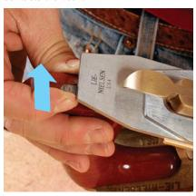
Move it to the center. Swing the lateral lever to bring the shaving closer to the center. If the shaving comes out on the left, move the adjuster to the left. Do the opposite if the shaving is on the right.
