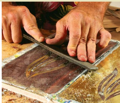
Continue with filing. A double-cut bastard mill file, held on edge, helps flatten the wood without gouging the metal.
