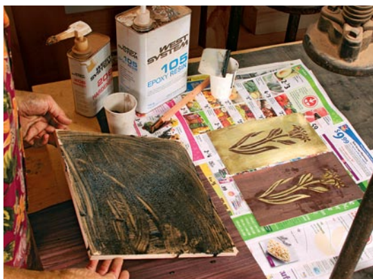
Fill in the blanks. After gluing paper to the show side of the panels, glue in the contrasting segments, working from the outside in.
