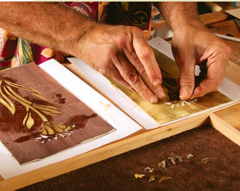
Fill in the blanks. After gluing paper to the show side of the panels, glue in the contrasting segments, working from the outside in.
