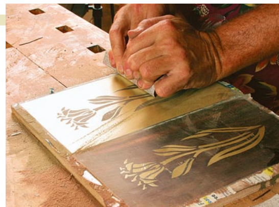
Sand by hand. Don't sand for too long in one place or use a powered sander. In either case you might heat the metal too much and break the glue bond.
