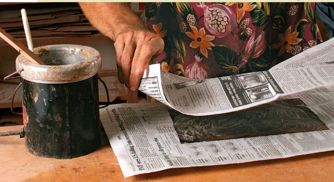
Reinforce the wood. To prevent small parts of the design from breaking along the grain when they are sawn, attach a piece of newspaper to the wood with hide glue.
