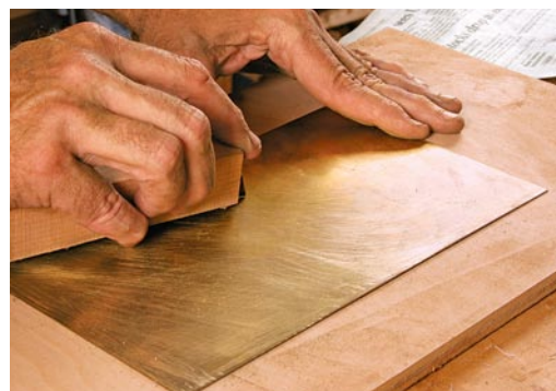
Abrade the metal. Use a piece of hacksaw blade inserted into a scrap of wood to scratch the glue face of the metal for a better bond with the substrate.
