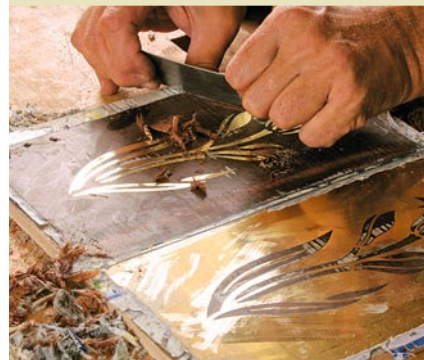
Start with a scraper. Use a cabinet scraper to remove the backing paper and begin bringing the wood flush with the brass.
