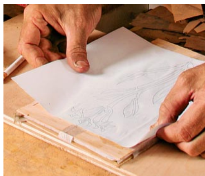
Attach the design. The last step before starting to saw is to attach the design to the wood-and-metal package with hide glue.
