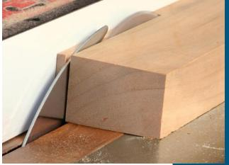
Choose low-profile when high-profile **can't be used.** For some cuts, the blade cover interferes with the operation. These include narrow rip cuts (left), and non-through-cuts like slotting (bottom left) and using a tenoning jig (bottom right). The low-profile knife stays just below the top of the blade, but gets you the same kickback protection as the high-profile system.
