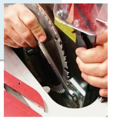
Four setscrews are used to adjust the knife-to-blade alignment on the Laguna. You only have to align it once; two socket-head screws secure the block to the arbor casting. To change knives, first remove the throat plate, then use a wrench (not included) to loosen a single hex bolt. Slip in the new knife and use the same
