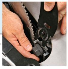
For knife alignment, the Grizzly uses a fixed knifeholding block. Metal shims are used to make side-to-side adjustments, but there's no way to adjust the knife if it's not parallel with the blade, short of bending it by hand. Ours needed bending, but I aligned it just fine. Both the low- and high-profile knives are removed by taking off the throat plate and loosening a single hex bolt.
