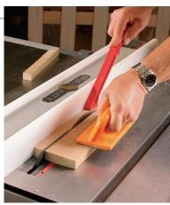
**Pinch protection.** A splitter or riving knife fills the kerf, so if the wood starts to close, it pinches the splitter or knife, not the blade, preventing kickback.
