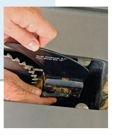
Like its cousin, the Jet saw, the Powermatic uses four setscrews to adjust the knifeholding block, and two more screws to lock the assembly once it's adjusted. To remove the low-profile knife, first take out the throat plate, then swing a lever handle to the
