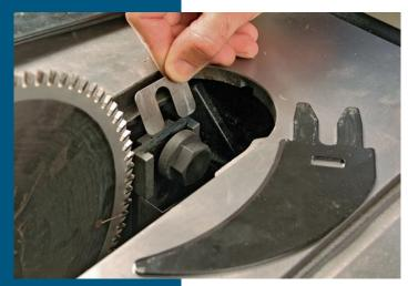
To work effectively, the knife must align with the blade. Even though it's essentially a one-time procedure, you don't want this adjustment to be a chore. Shims (above) take more time; screws (right) provide control and simplicity.
