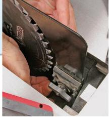
The Steel City saw uses four setscrews to adjust the knife-to-blade alignment. To remove a knife, lift out the throat plate and turn a springloaded locking knob about 11/2 times. Once loosened, pull the knob and remove the knife. I'd have liked a bigger knob,
