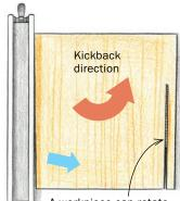
A workpiece can rotate away from the fence and into the rear teeth of the blade, hurling the workpiece like a Frisbee.
