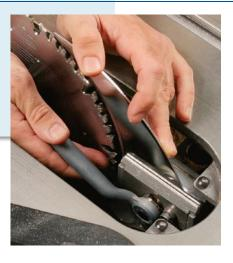
A pair of socket-head screws allows only side-to-side blade alignment. Any lack of parallelism between the knife and blade (our saw didn't have any) requires hand-bending the knife. Not high-tech, but it will work. With the throat plate removed, the knives
