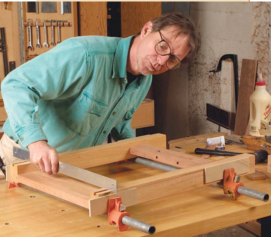
Assemble the table sides. Apply glue to the tenon cheeks and the mortise walls and then assemble each side separately, checking to make sure they go together square and true.
