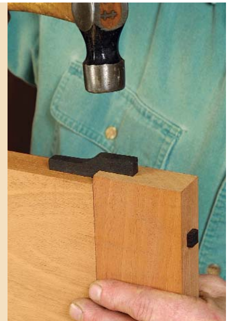
Apply the ebony plugs and end caps. Glue the ebony end cap only to the tabletop panel so that it can move freely in the breadboard end.
