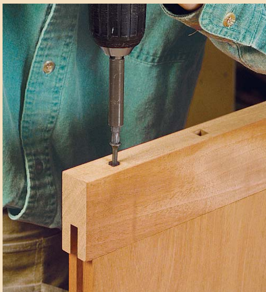
Drive screws through the breadboard ends. The holes on either side of center should be elongated to allow the panel to expand and contract.
