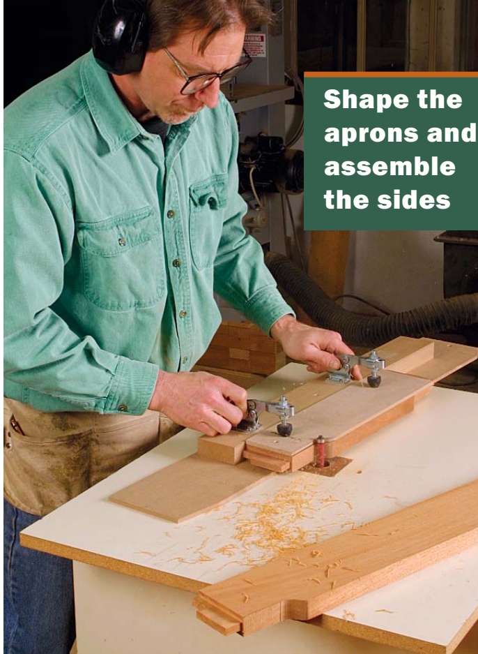
Cut the cloud lift with a template and router table. Rout the cloud-lift motif on the aprons after cutting and fitting the apron tenons in the leg mortises.
