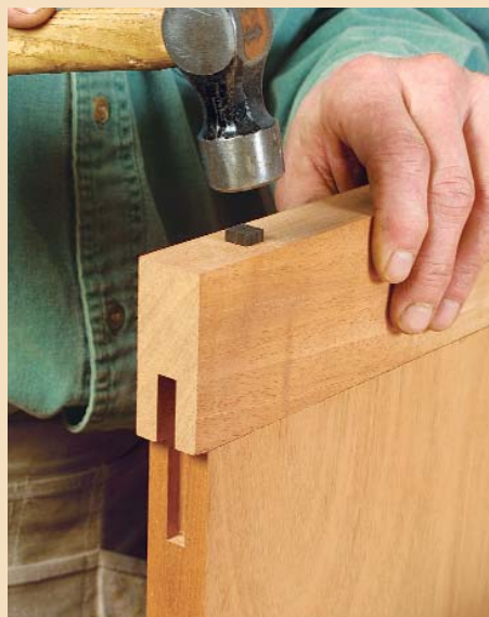
Apply the ebony plugs and end caps. Glue the ebony end cap only to the tabletop panel so that it can move freely in the breadboard end.
