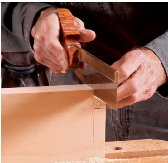
Arched cutout creates two feet. Stay close to the layout line with the coping saw, then fair the curve with sandpaper attached to the curved offcut.
