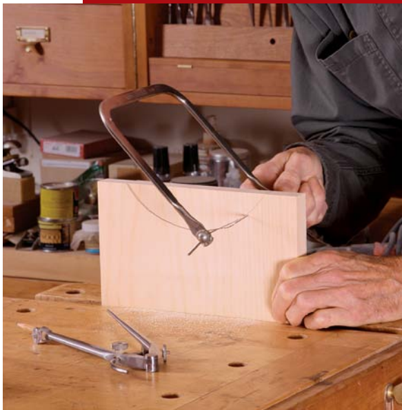
Arched cutout creates two feet. Stay close to the layout line with the coping saw, then fair the curve with sandpaper attached to the curved offcut.
