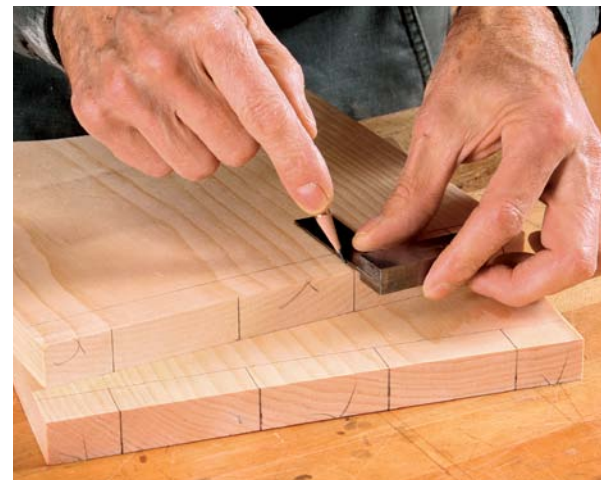
Then mark the width. Measure in from each edge to mark the width of each tenon. Use a square to carry the layout lines from each mark across the top edge and down to the baseline.
