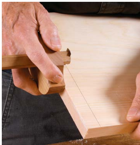
Scribe the tenon length. Set a marking gauge to the thickness of the top and use it to create a baseline for the tenons on both faces and ends of each leg.
