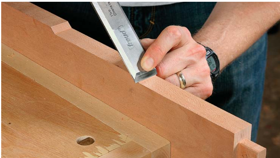
Clean up with a chisel. It's the best tool for the small transition. For the horizontal surface, use a block plane, switching to the chisel near the corner where the plane can't reach.
