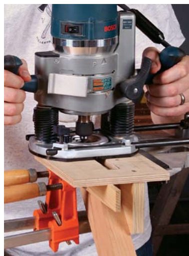
Mind the edge guide. Use a spiral bit, and pull the router toward the outside of the joint to keep the edge guide tight.
