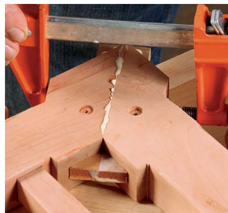
Clamp the miters last. The horns left on the leg and top rail provide a square clamping surface, so there's no problem getting enough pressure on the joint to create a tight glue line.
