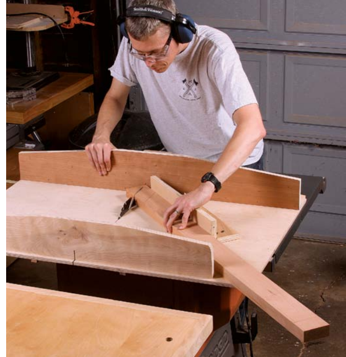
Use a sled for the miters. Your miter gauge won't hold these big pieces as securely or give you as accurate a miter.
