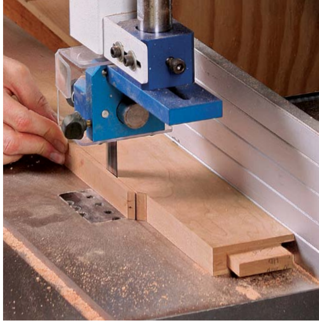
Stopped cuts create the clouds. Use the fence for the long horizontal sections, and cut the angled transitions freehand.
