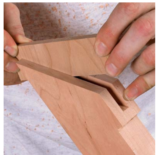
Grain direction matters. Cut off the spline across the grain, so it will move in the same direction as the post and top rail and won't push the joint open.
