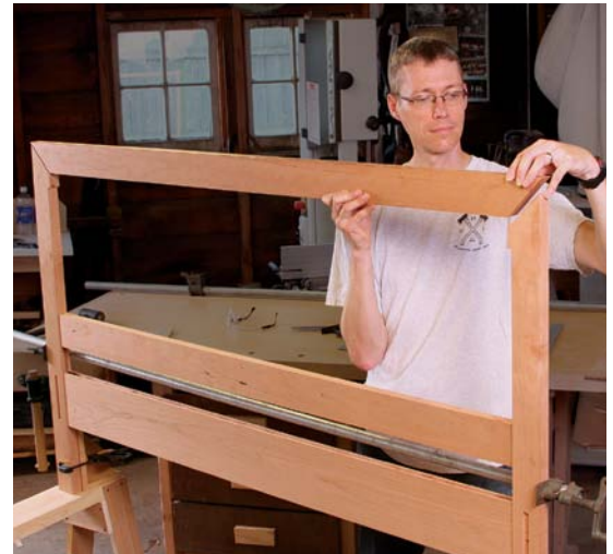
Use a sled for the miters. Your miter gauge won't hold these big pieces as securely or give you as accurate a miter.
