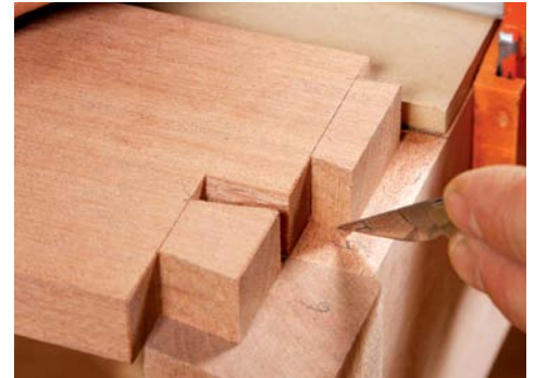
Double dovetail. After cutting two tails on the end of the rail, transfer their locations to the leg and apron. Make the sockets and fit the joint.
