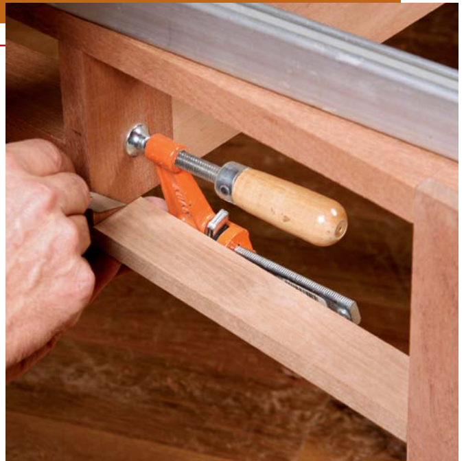
Make a template first. Use a piece of scrap, and trim the ends at 9° so it fits between the leg and end cap.
