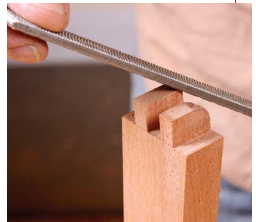
Round over the top of the tenons. This will let you pivot the piece into place later.
