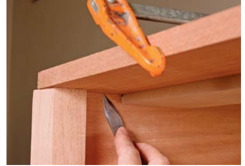
Mark the joint. Center the top rail, clamp it to the spacer, and mark a shoulder line by scribing around the leg and apron.
