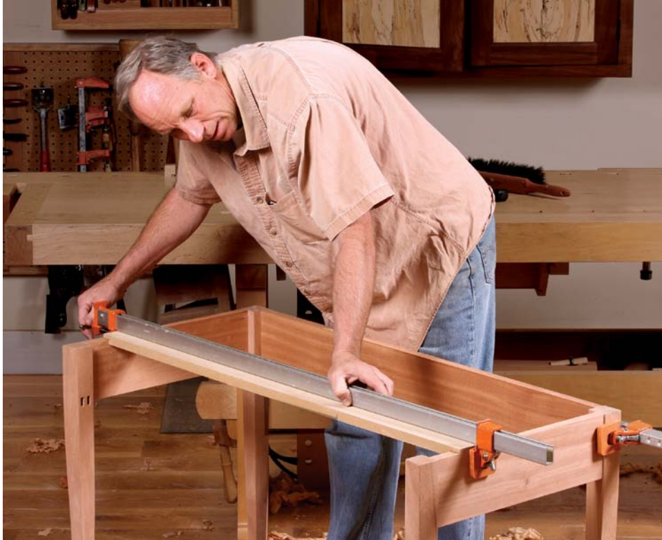
Dry-assemble the base. Clamp the sides to the back apron. A spacer up front keeps the base square. Place its front edge 3\frac{3}{8} in. from the leg's front, as a reference for locating the top rail.
