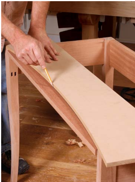
Finish the rail. Dry-fit it and scribe the arc, lining it up with the legs. Now lay out the double mortises for the drawer divider end caps. Simplify the mortising using a spacer between the rail and fence when making the second mortise (center). Rough out the curve on the band-saw, then rout the rail flush to the template (right).
