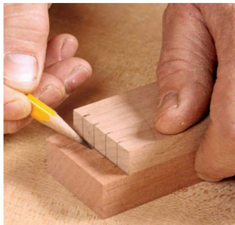
Lay out the joints on the rail. Use the template to lay out the shoulders and tenons.
