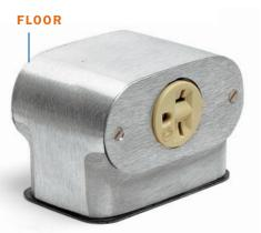
Another way to bring power to the middle of your shop is to use a monument-style receptacle. This type avoids the problems of a flush-mounted receptacle, which include dust clogging and possible shorts from metal objects.
