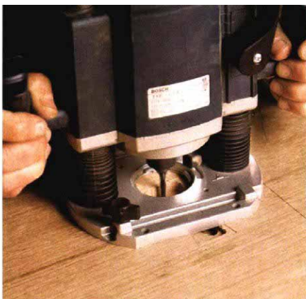
3) Plunge-rout the mortise with a \frac{1}{4} -in. straight bit.
