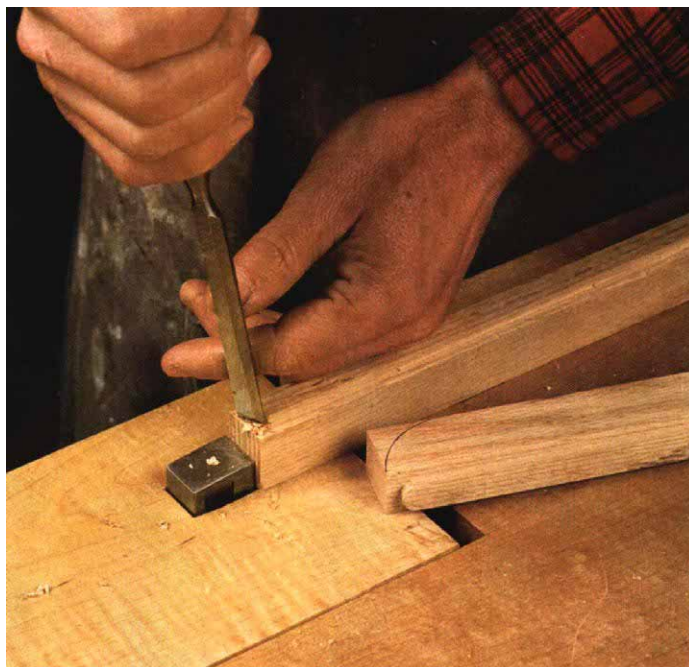
Rounding off the dovetail tenons —After shaping the upper rails' dovetails on his router table, the author uses a \frac{1}{2} -in. straight chisel to trim the ends. Rounding the ends ensures that the dovetail tenons fit the stopped grooves in the underside of the top. Next Vogt will bandsaw the curve marked on the rail.
