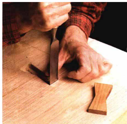
4) Pare to the line, and clean up the corners with chisels.
