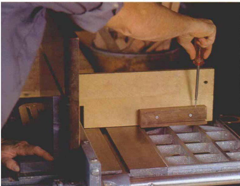
The auxiliary fence can be adjusted so it's exactly 90^\circ to the saw table by means of a spring-like block screwed to the fence's brace. A kerf partially across the block provides enough flexibility to tip the fence by driving a single screw in or out.
