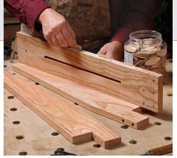
**Fixed column is biscuited.** After notching the outside pieces to fit tightly onto the base, attach them to the center piece.
