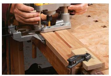
**Rout the slots.** The fixed and sliding columns have <sup>3</sup>%-in. bolt holes and <sup>3</sup>%-in. slots, which must line up precisely. Drill the holes first, and then use them to set up the router for the long slots.
