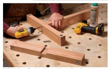
**Build the base.** The base pieces are joined with shallow dadoes, long screws, and glue.
