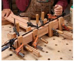
strong bridle joint at the base. That joint is also glued and screwed.
