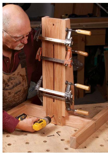
**Glue and screws anchor the column.** Screw in from the front and back to attach the fixed column to the base.
