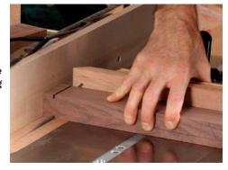
Use the mortises as a map. Lay the apron on the leg to mark the inside cheek cuts.
