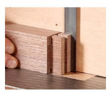
**Outside cheeks next.** Coleman removes most of the waste on the outer cheeks with the bandsaw.
