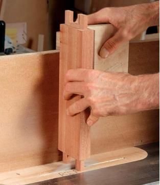
Cut and flip. After cutting the tenon cheeks and shoulders, Coleman uses a shopmade tenoning jig (see drawing, left) and a flat-top rip blade to excavate between the stacked tenons. Make a cut and then flip the apron end for end to make the same cut on the opposite end (left). Then adjust the fence and repeat. When you're close, check the fit (below) and trim where needed.
