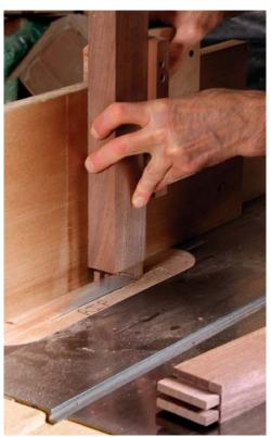
**Final cuts.** Use a tenoning jig and a flat-top rip blade to skim the outside cheeks. Check the fit as you go.
