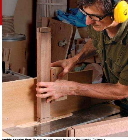
**Inside cheeks first.** To remove the waste between the tenons, Coleman uses a flat-top rip blade and a tenoning jig, cutting about  $^{1}/64$  in. proud of the shoulder. He pares to the line later with a narrow chisel.
