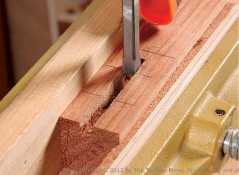
racking force could cause the leg to split. Also, unless there's a haunch, set the tenons at least 3/8 in. below the top of the leg. Any closer, and that weak end grain area would not have enough meat to resist leverage from the top of the tenon.
