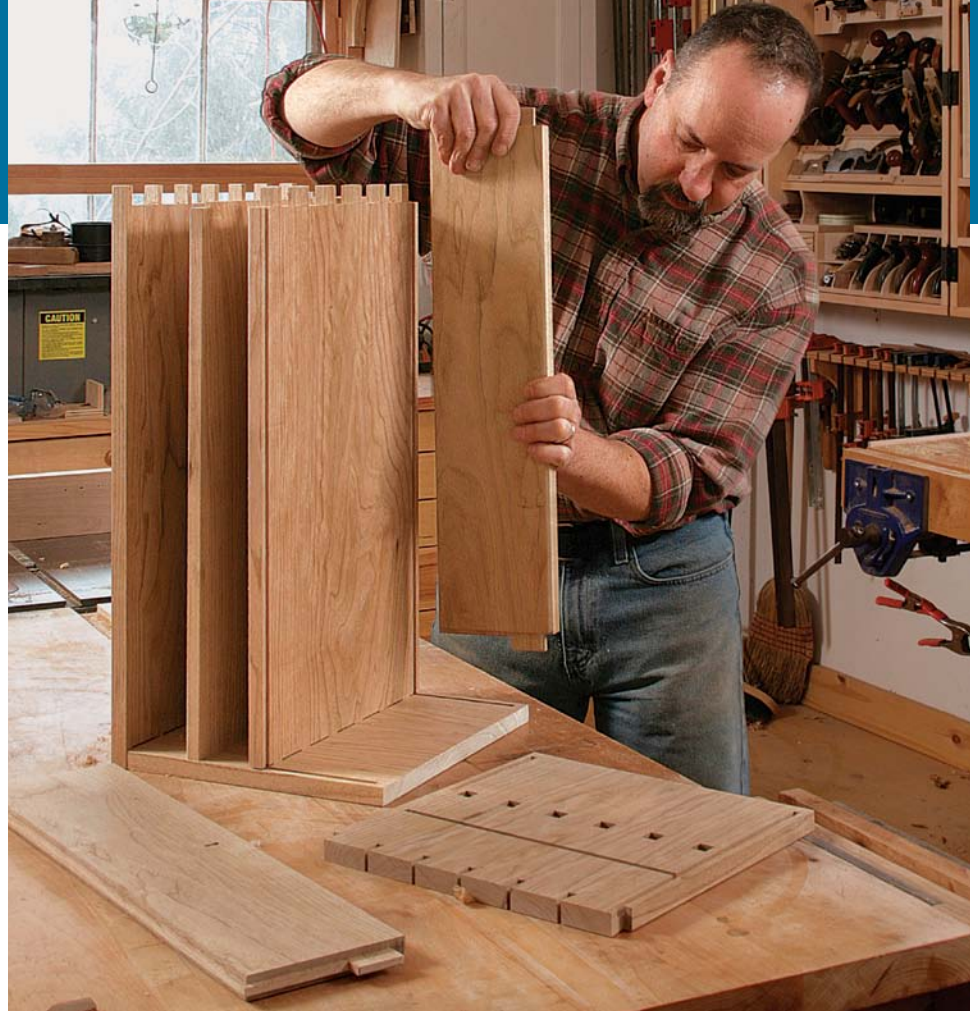
One big glue-up. Unfortunately the case glue-up can't be broken into smaller sub-assemblies. So do a dry run (above) to reduce some of the stress and avoid any surprises once the glue is on. For the actual glue-up, use plenty of clamps to bring the claps together. Then put glue in the slots in the shelf tenons and drive wedges in place (left).
