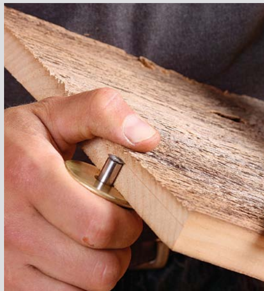
Rabbit the shelves to fit. The jointed bottoms of the shelves create a reference face for scribing perfectly even rabbets (left). Tetrauilt rabbets the shelf using a thick piece of wood to guide a rabbeting block plane (right).
