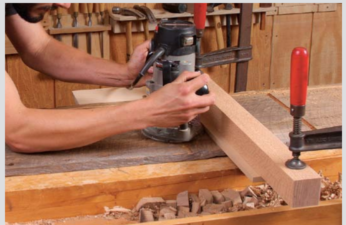
A T-square for dados. Square the jig from the back edge and then use a thick caul to clamp the whole board flat.
