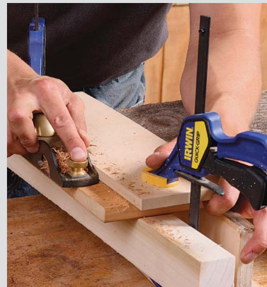
Rabbit the shelves to fit. The jointed bottoms of the shelves create a reference face for scribing perfectly even rabbets (left). Tetrauilt rabbets the shelf using a thick piece of wood to guide a rabbeting block plane (right).
