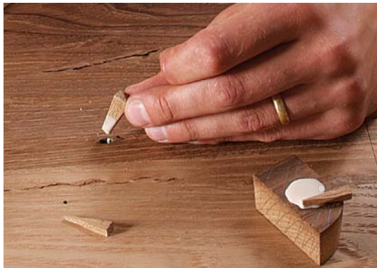
Plug holes with scrap. Chisel random-shaped pegs from offcuts and glue them into nail holes or worm holes (left). Then trim them flush (above).
