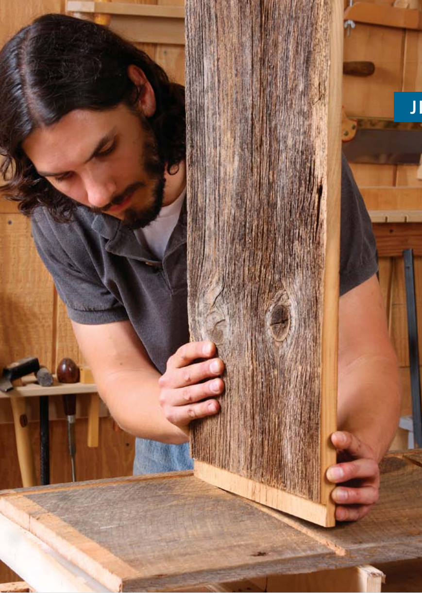
A T-square for dados. Square the jig from the back edge and then use a thick caul to clamp the whole board flat.
